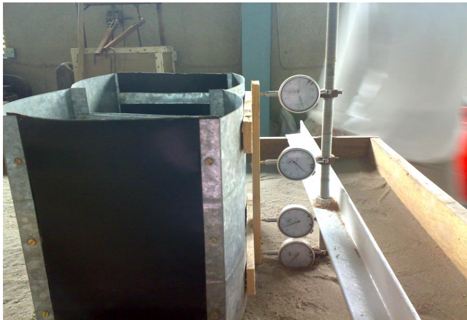
Fig. (3-18): Steel shaft carry four dial gages
