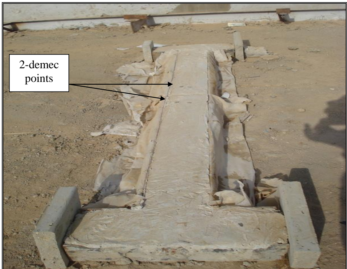
Plate(3-10) Free shrinkage measurement (I-shape mold)
