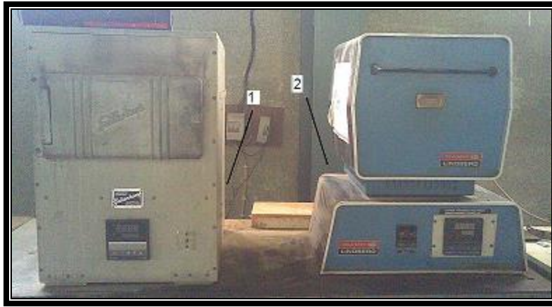
Figure (4.4) Equipment of electric furnaces. 1. (REC TRADEUAR) type. 2. (SOLA BASIC 51222) type.
