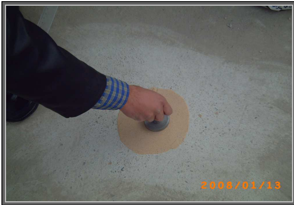
Plate (3.1): Volumetric Method.
