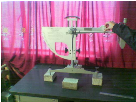
c. The pendulum was raised and clamped horizontally in place.
