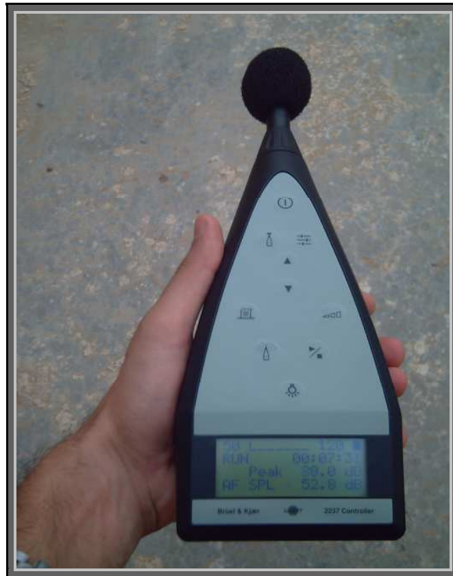
Figure (3.5) : Sound measurement sound level meter (SLM).
