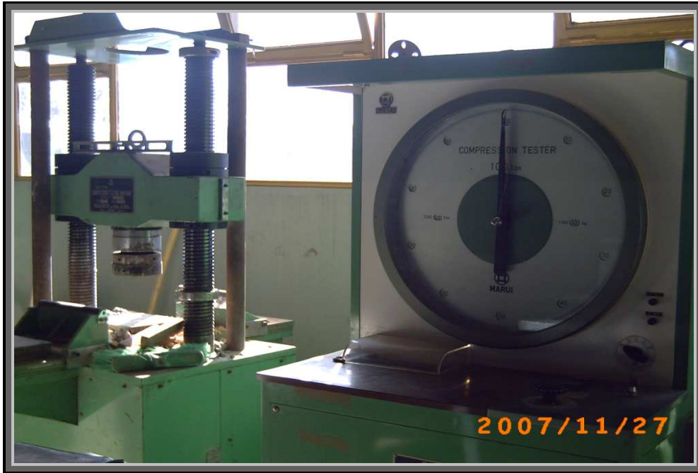
Plate (3.3) : Compressive Strength Test.
