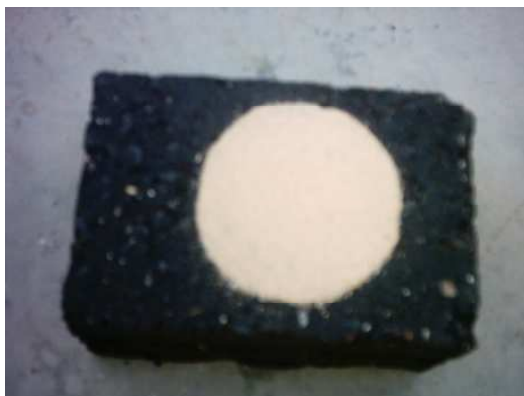
e. Sand being spread to fill surface voids.
