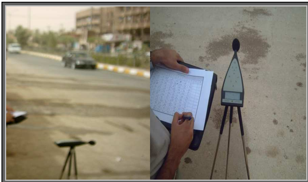
Figure (3.6) : Typical measurement set up for SPB measurement
