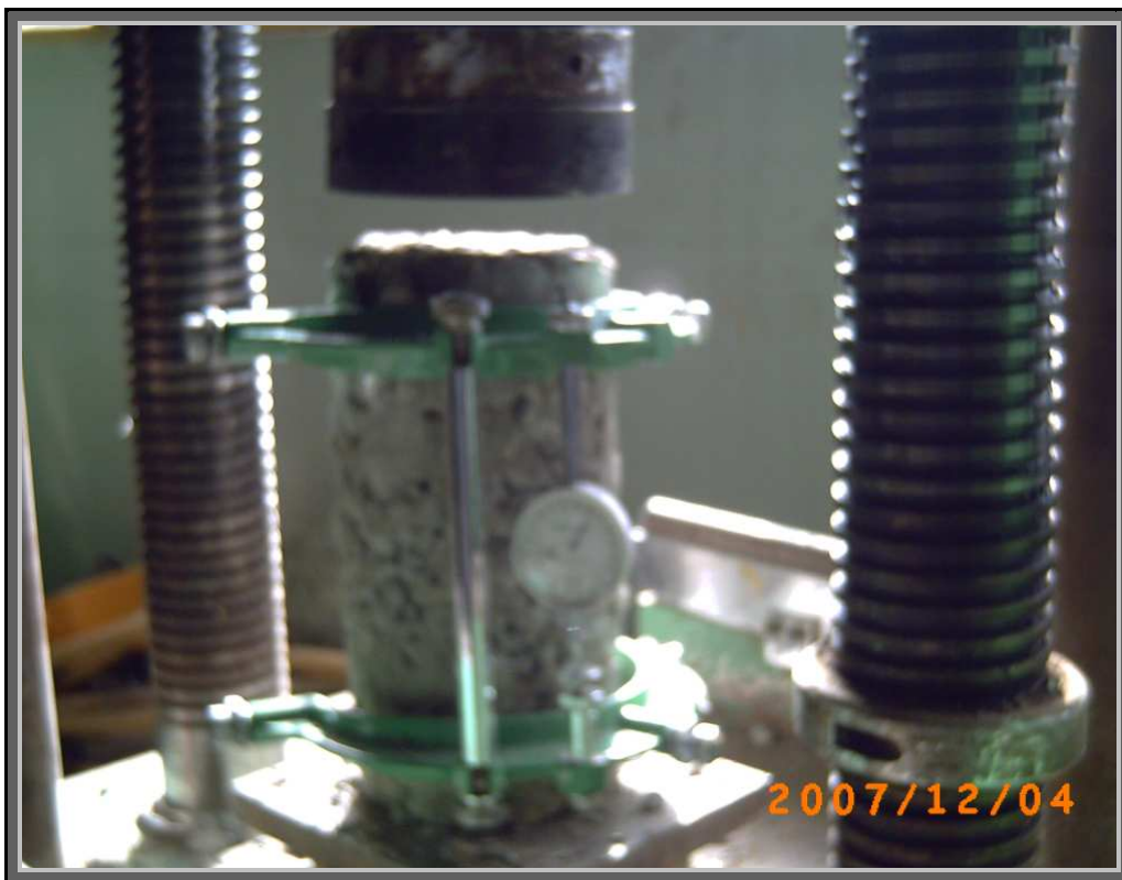
Plate (3.4) : Static Modulus of Elasticity Test.
