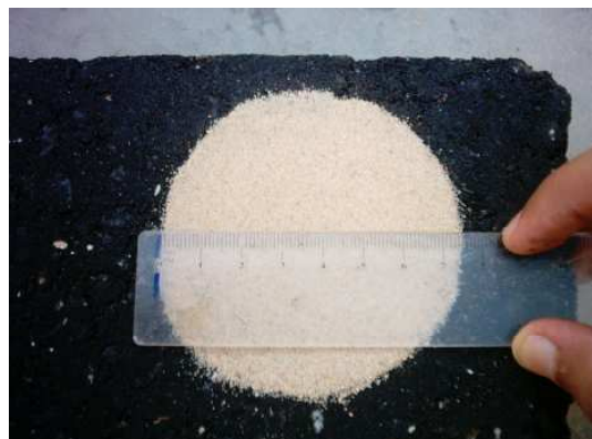
f. Measuring diameter of Sand circle.
