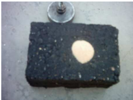
c. Sand poured onto pavement.
