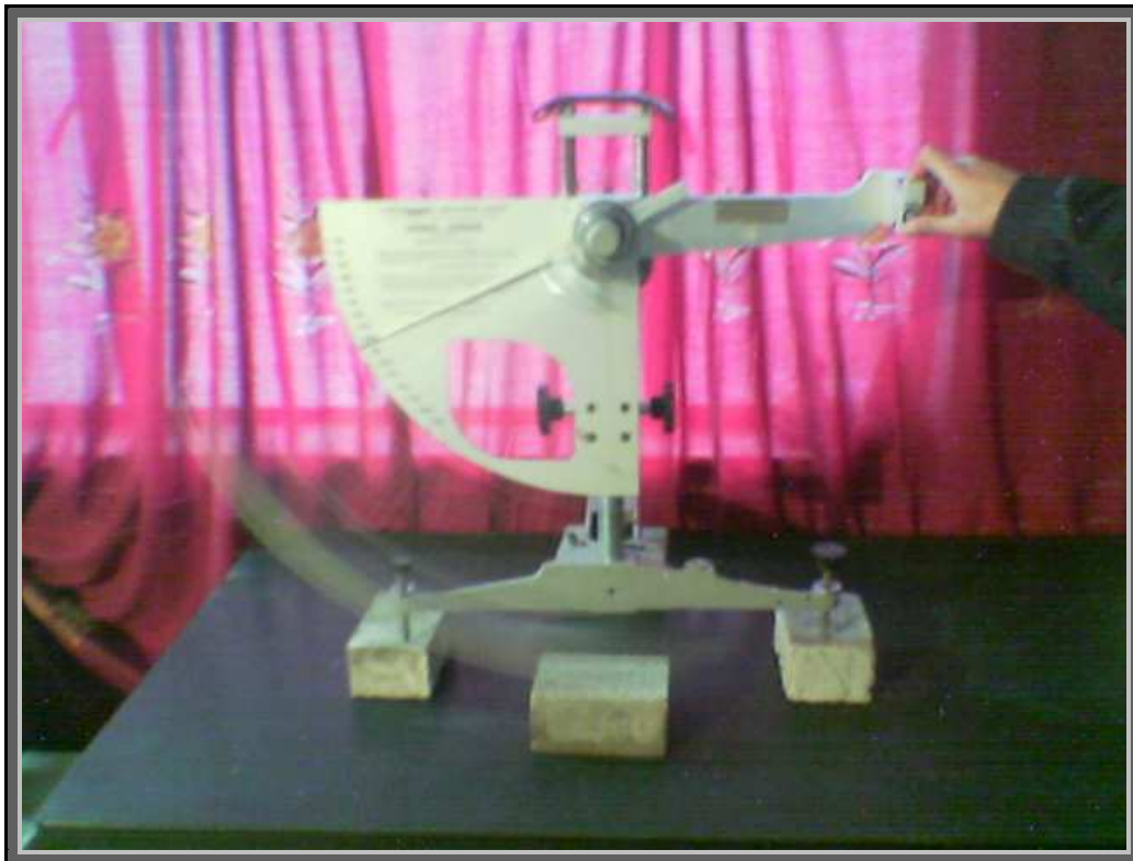
Plate (3.2) : The British Pendulum Test.
