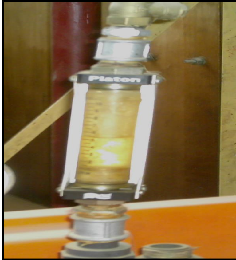
Figure (4-4) water flow meter.
