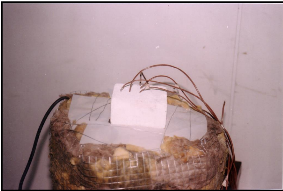
Fig (4-5) MgO test sample with heater
