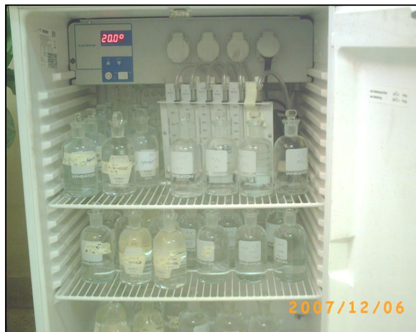
Fig.(4-10) :Samples of BOD 5 Inside the Incubator
