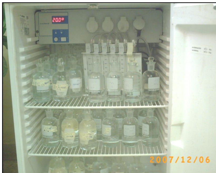
Fig.(4-10) :Samples of BOD 5 Inside the Incubator
