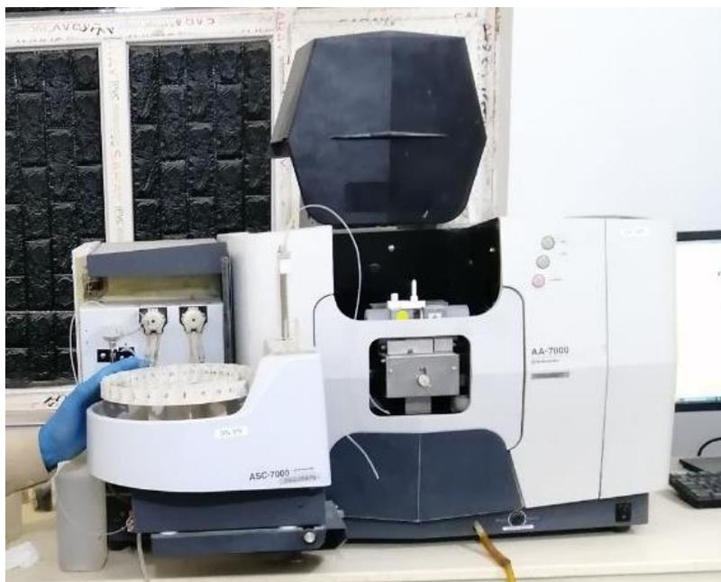
**Figure 3.5: Atomic Absorption Spectrophotometer**
