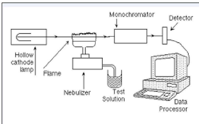
**Figure 3.6: Atomic Absorption Meter Parts Diagram [35].**
