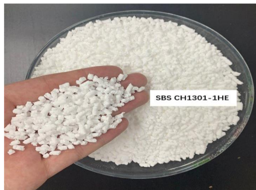
Figure 1: Styrene Butadiene Styrene Copolymer Asphalt Modifier Material Pellet
