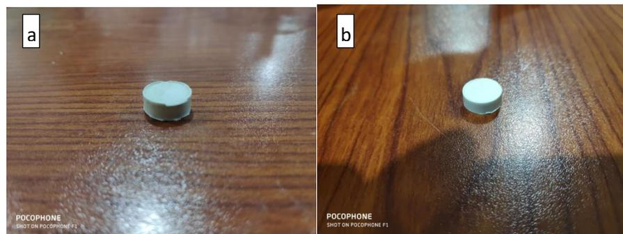
**Figure1.** Samples (a) before sintering, (b) after sintering with surface finishing (grinding and polishing).
