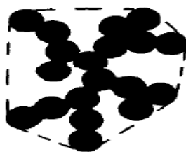
Fig. 2: Schematic of a carbon black aggregate consisting of fused primary particles. The dotted line (a surface in 3D) depicts the volume [6]
