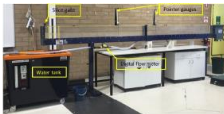
Figure 1. Hydraulic flume details
