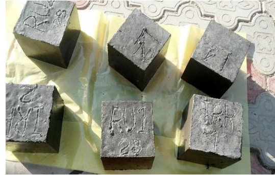
Fig (3): show the concrete samples after the process of curing
