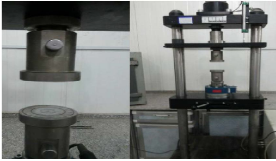
Figure (4) Compression strength machine.
