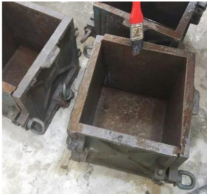
Fig (2): lubrication of mold
