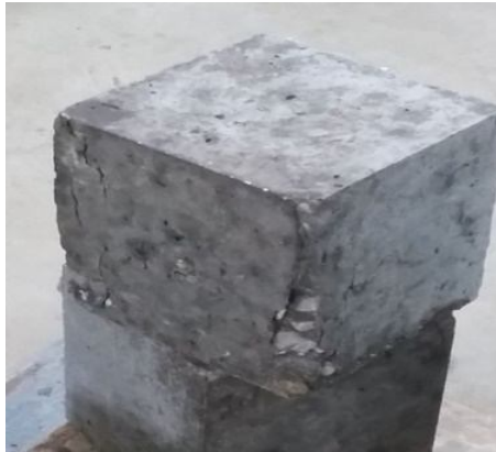
Fig (5): shows the concrete cubes after the compression test with no access to the failure condition
