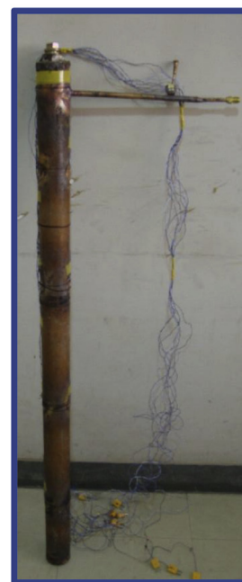
Fig. 5. (A) schematic diagram of cooling rate sensor. (b): photograph of cooling rate sensor.
