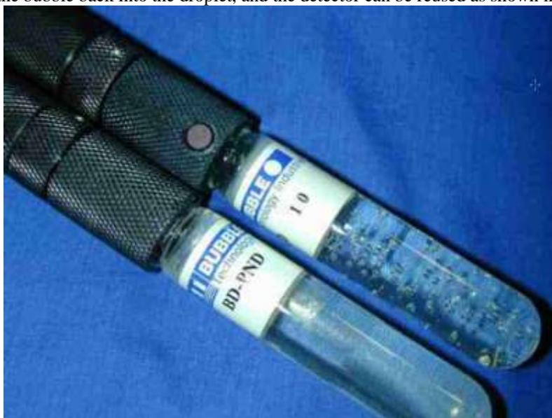
**FIGURE 4.** Super-heated emulsion-based detector (DLJ)
