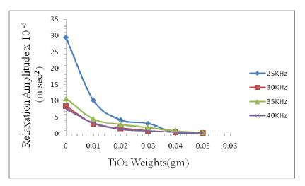
Fig. (11) The relaxation amplitude due to the TiO2 Weights
