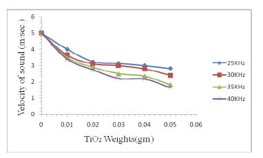
Fig. (2) The velocity of sound due to the TiO2 Weights
