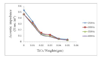
Fig. (4) The acoustic impedance due to the TiO2 Weights
