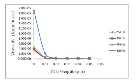
Fig. (10) The viscosity due to the TiO2 Weights
