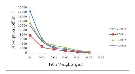
Fig. (7) The absorption coefficient due to the TiO2 Weights
