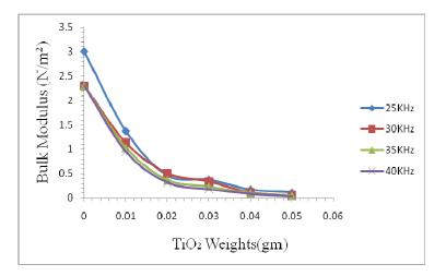
Fig. (3) The bulk modulus due to the TiO2 Weights
