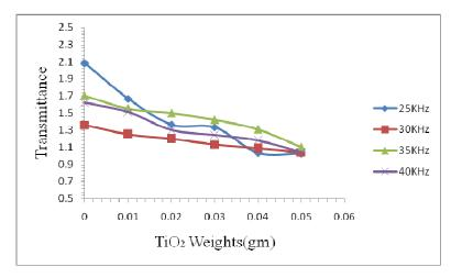
Fig. (6) The transmittance due to the TiO2 Weights
