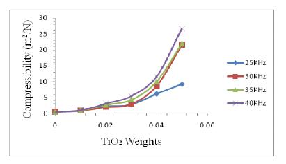
Fig. (5) The compressibility due to the TiO2 Weights
