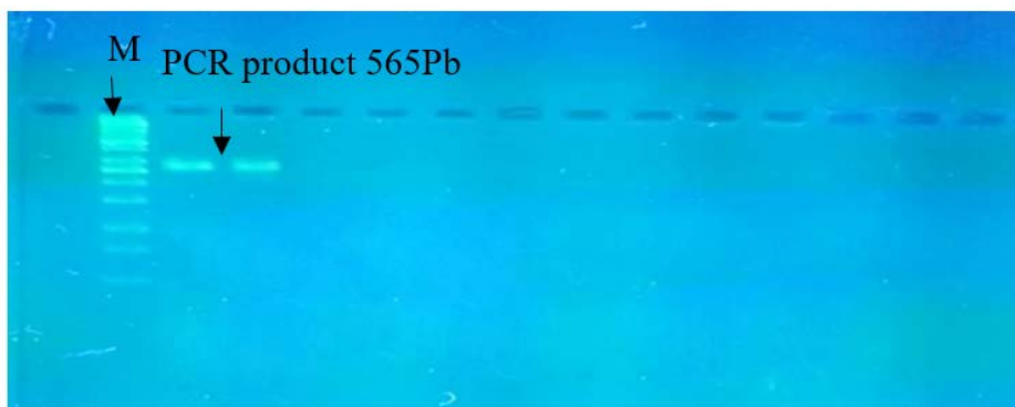
Fig. 2. PCR product, the band size of 565 bp. The product was electrophoresis on 1.5% agarose at 5 volt/cm 2 . Also, 1x TBE buffer for 1.5 h, DNA ladder (100), lane (1 to 2) PCR product of band size 565 bp, visualized under UV light
