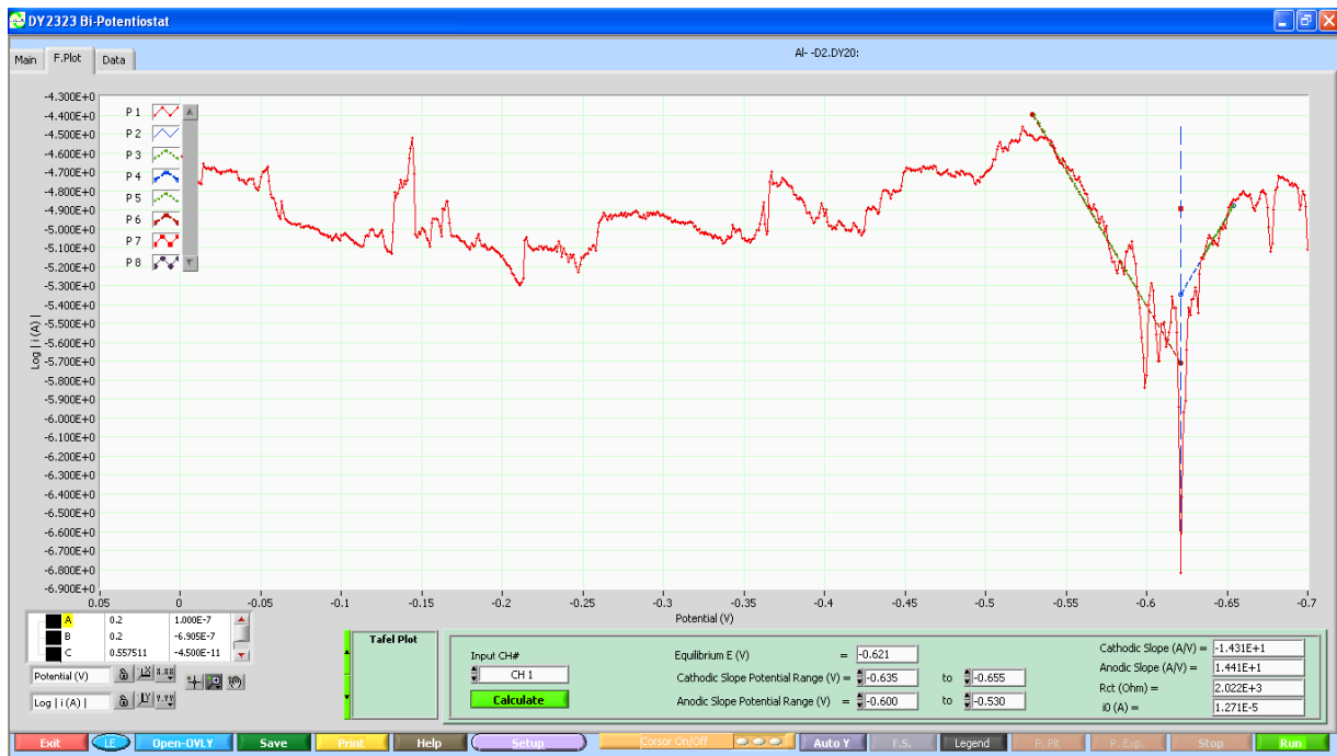
Fig. (5) polarization curve of amalgam D in synthetic saliva at 37\pm 1 C°.
