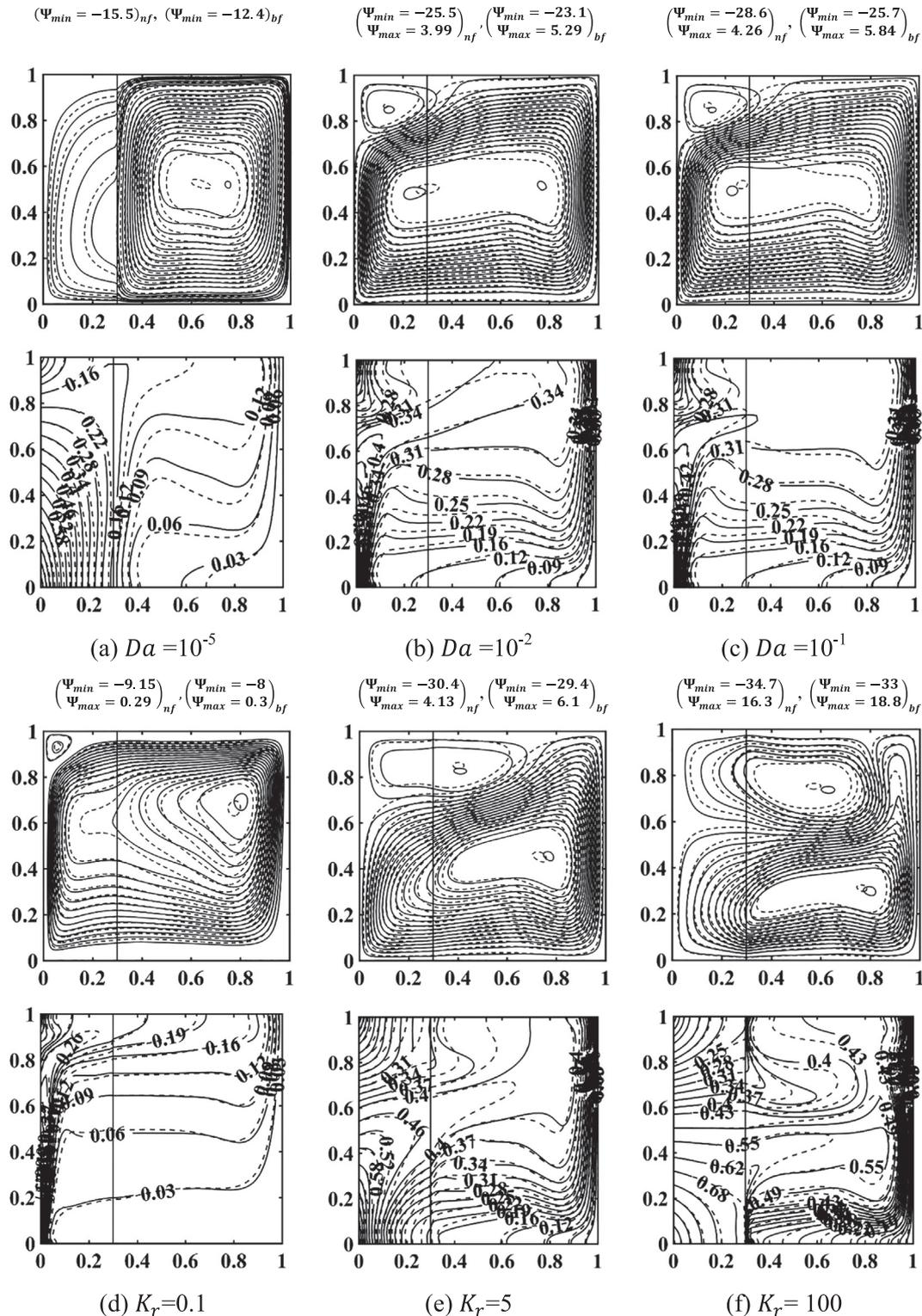
**Fig. 7.** Streamlines (upper row) and isotherms (lower row) for case 1 with  $\phi = 0$  (solid lines) and  $\phi = 0.1$  (dashed lines) at different dimensionless parameters. (a–c)  $Da$  effect when  $Ra = 10^6$ ,  $S = 0.3$  and  $K_r = 1$ , and (d–f)  $K_r$  effect when  $Ra = 10^6$ ,  $Da = 10^{-3}$  and  $S = 0.3$ .
