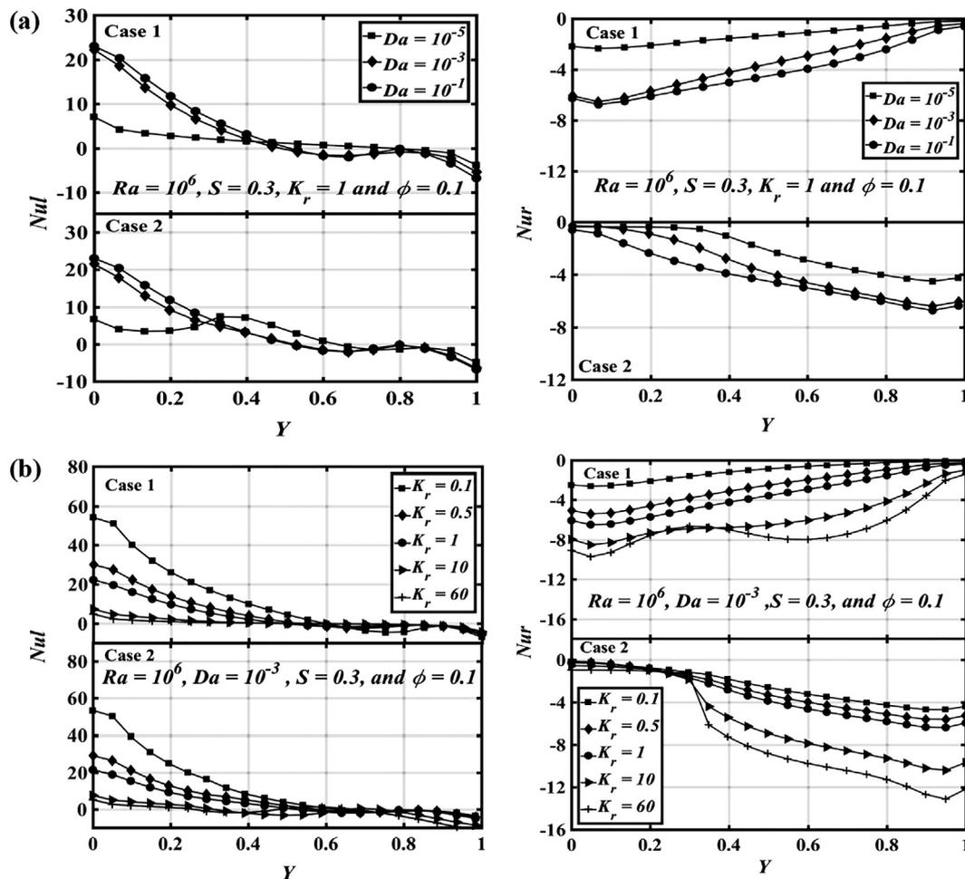
Fig. 12. Variation of the local Nusselt number along the left hot wall (left column) and the right cold wall (right column) with different dimensionless parameters (a)  $Da$  effect and (b)  $K_r$  effect.
