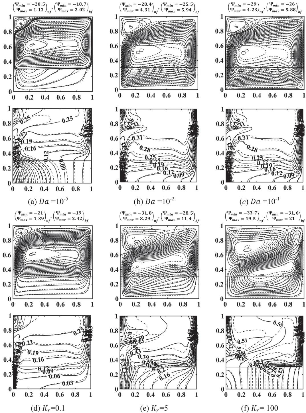
**Fig. 9.** Streamlines (upper row) and isotherms (lower row) for case 2 with  $\phi = 0$  (solid lines) and  $\phi = 0.1$  (dashed lines) at different dimensionless parameters, (a–c)  $Da$  effect when  $Ra = 10^6$ ,  $S = 0.3$  and  $Kr = 1$ , and (d–f)  $K_r$  effect when  $Ra = 10^6$ ,  $Da = 10^{-3}$  and  $S = 0.3$ .
