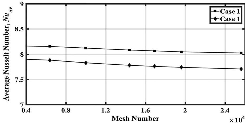
Fig. 5. Grid testing for the average Nusselt number at different mesh numbers.
