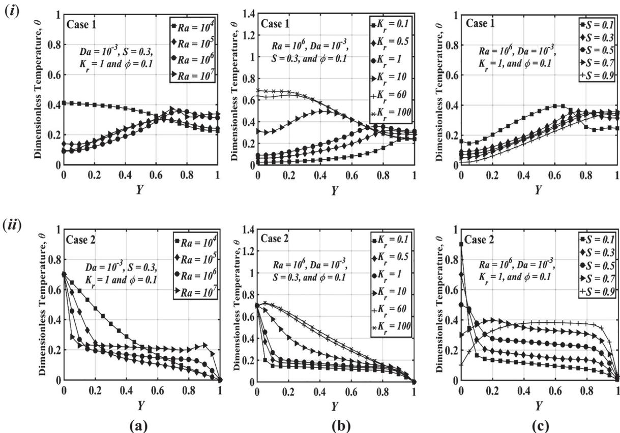
Fig. 11. Local distribution of dimensionless temperature along the interface line for (i) case 1 and (ii) case 2 with different dimensionless parameters (a)  $Ra$  effect, (b)  $K_r$  effect, and (c)  $S$  effect.
