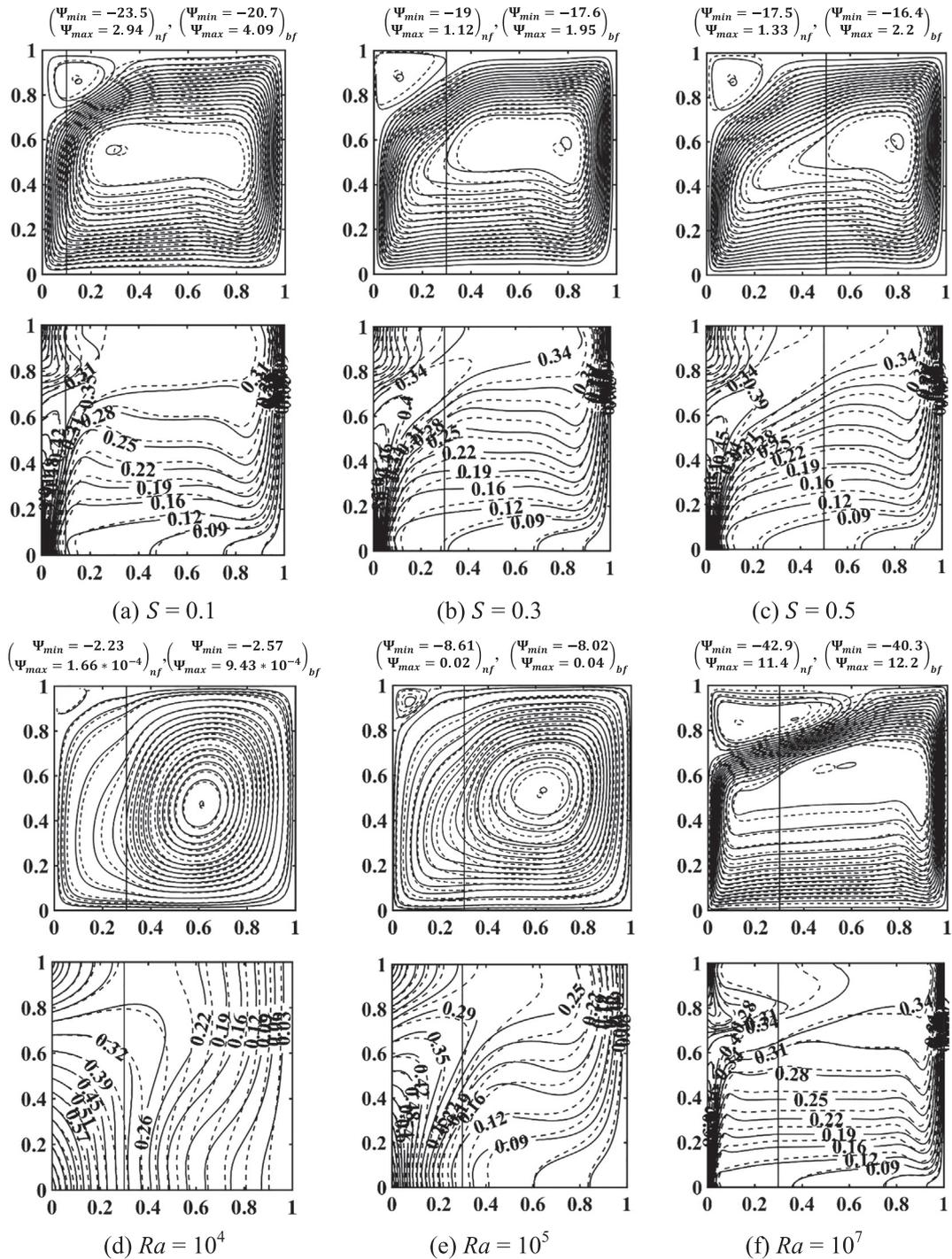
**Fig. 6.** Streamlines (upper row) and isotherms (lower row) for case 1 with  $\phi = 0$  (solid lines) and  $\phi = 0.1$  (dashed lines) at different dimensionless parameters, (a–c)  $S$  effect when  $Ra = 10^6$ ,  $Da = 10^{-3}$  and  $K_r = 1$ , (d–f)  $Ra$  effect when  $Da = 10^{-3}$ ,  $S = 0.3$  and  $K_r = 1$ .
