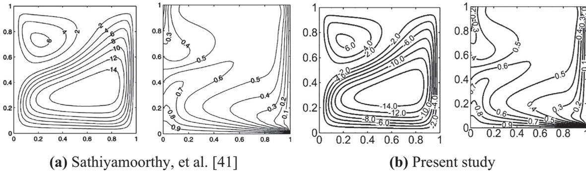
**Fig. 3.** Streamlines (left) and isotherms (right), for the case  $\theta = 1 - y$  on the left wall and  $\theta = 0$  on the right wall and adiabatic top and bottom walls at  $Ra = 10^6$ ,  $Da = 10^{-5}$  and  $Pr = 0.7$ . The left panel corresponds to (a) Sathiyamoorthy et al. [41] and the right panel corresponds to (b) the present study.
