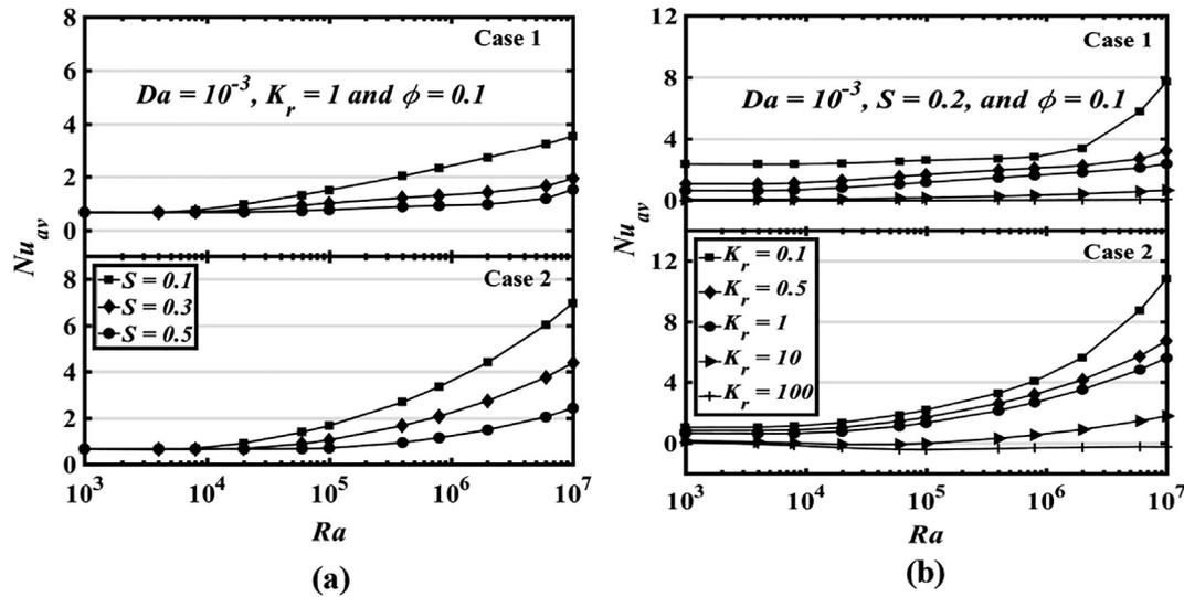
**Fig. 13.** Variation of the average Nusselt number versus  $Ra$ , (a)  $S$  effect and (b)  $K_r$  effect. In each plot, the upper panel corresponds to case 1, and the lower panel corresponds to case 2.
