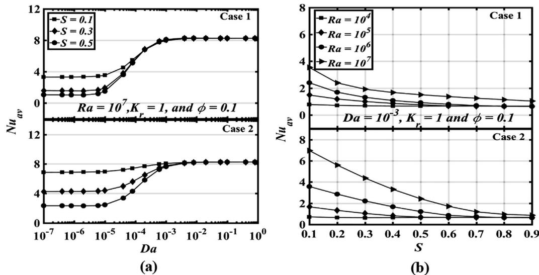
**Fig. 14.** Variation of the average Nusselt number with (a)  $Da$  number for different  $S$  and with (b) porous layer thickness  $S$  for different  $Ra$ . In each plot, The upper panel corresponds to case 1, and the lower panel corresponds to case 2.
