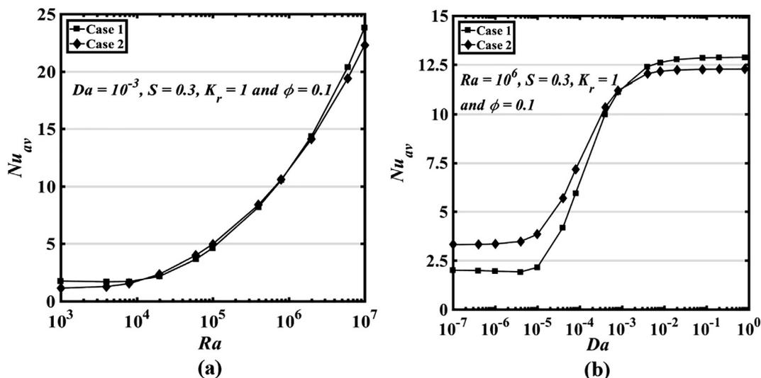
Fig. 15. Variation of the average Nusselt number with (a)  $Ra$ , and (b)  $Da$ , for case 1 and case 2 with linear heating on the left vertical sidewall.
