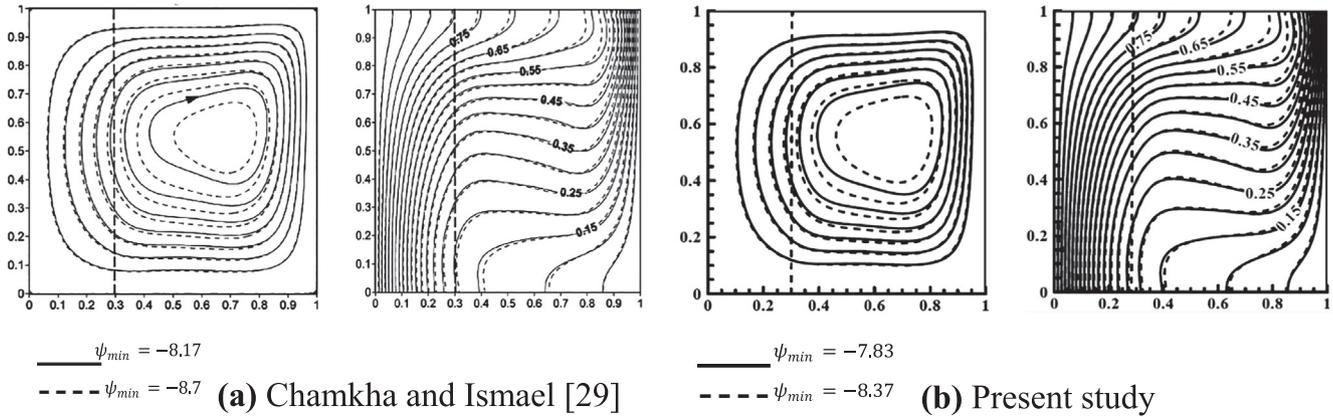
**Fig. 2.** Streamlines (left) and isotherms (right), for a square cavity with uniform hot left sidewall and cold right sidewall and adiabatic top and bottom walls at  $Ra = 10^5$ ,  $Da = 10^{-5}$ , aspect ratio = 1, porous layer thickness = 0.3,  $\phi = 0$  (solid lines) and  $\phi = 0.05$  (dashed lines). The left panel corresponds to (a) Chamkha and Ismael [29] and the right panel corresponds to (b) the present study.
