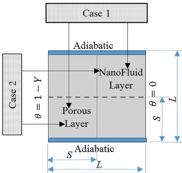
Fig. 1. Physical domain of vertical (case 1) and horizontal (case 2) directions of the composite nanofluid-porous medium layers.
