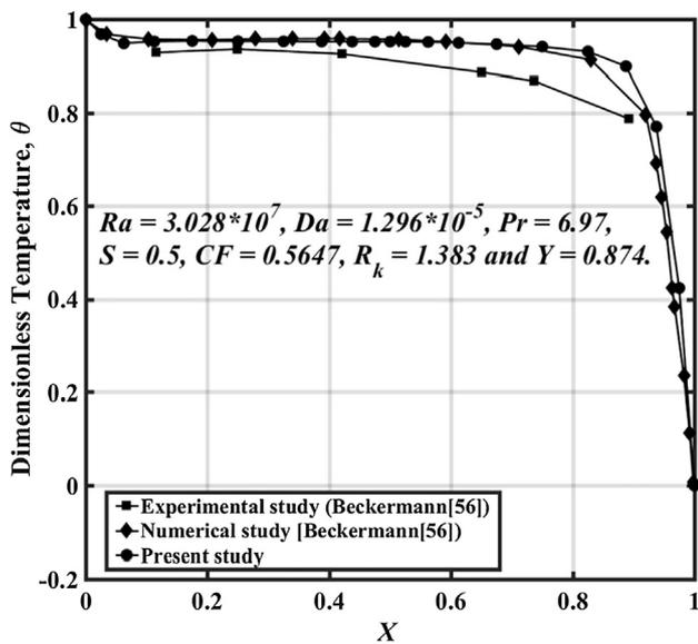
**Fig. 4.** Validation of numerical and experimental results presented by Beckermann et al. [56] with the present result.
