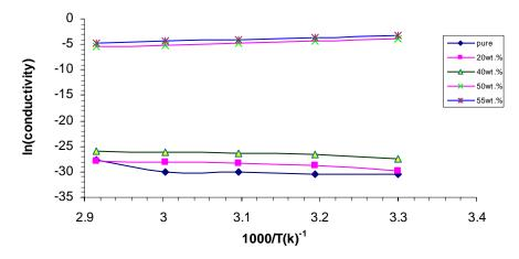
The concentration increasing of Zinc less the result of the activation energy as shown in the figure (5) of PVC- Zn composites for ( $\Phi < \Phi_c$ )which is a reasonable support for the above discussion [Ahmed and Zihilif,1992].
