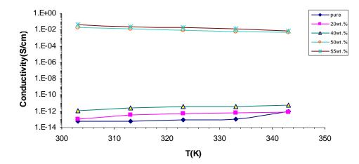
Figure (4) shows the relationship between the ln(conductivity) and inverted absolute temperature of the PVC-Zinc composites, using equation  $\sigma = \sigma_0 \exp(-E_a/k_BT)$  was calculate activation energy, the high activation energy values for neat sample and low Zinc concentration sample can be attributed to the thermal movement of the ions and molecules, whereas the low activation energy
