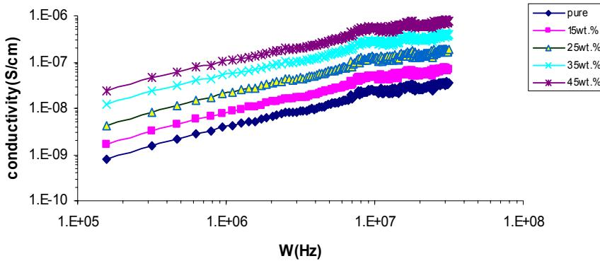
The increasing of A.C electrical conductivity in high frequency region can be related to the electronic polarization as well as to the hopping of charge carrier over a small barrier height. The figure also indicates that  $\sigma_{A,C}$  is increasing with increasing Al<sub>2</sub>O<sub>3</sub> wt.% content, a result which supports the suggestion of hopping of charge carrier conduction mechanism [Hamzah M.*et al*,2008].
