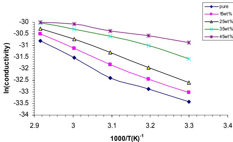
The concentration increasing of Al<sub>2</sub>O<sub>3</sub> less the result of the activation energy as shown in the figure (5) of PMMA-Al<sub>2</sub>O<sub>3</sub> composites which is a reasonable support for the above discussion [Ahmed and Zihilif,1992].
