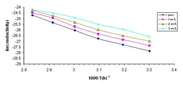
The addition of low concentrations creates local energy levels in the forbidden energy gap which act as traps for charge carriers, which move by hopping among these levels. By increasing the calcium oxide concentrations, the activation energy decreases as a result of the increase of local centres [6], as shown in figure(4).
