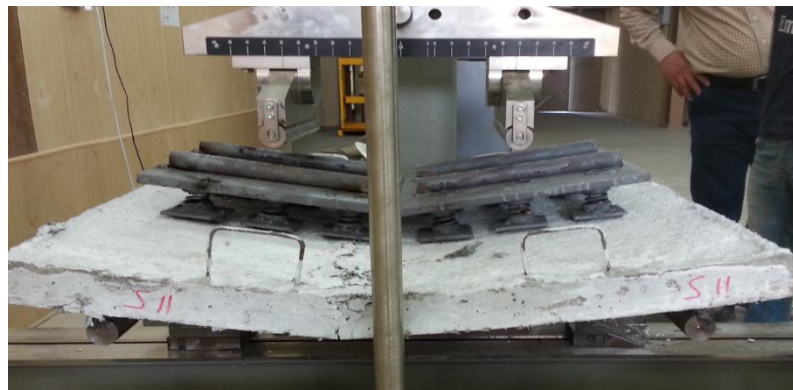
Figure 11. Ductile failure of slab PVC-60.
