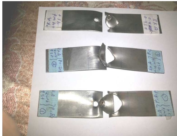
Figure 18a: Effect the Weld Current on the Failure Modes, (B): Effect the Weld Time on Fracture Mode, (C): Effect the Force Electrode on the Fracture Mode of LCS/304LSS RWS
