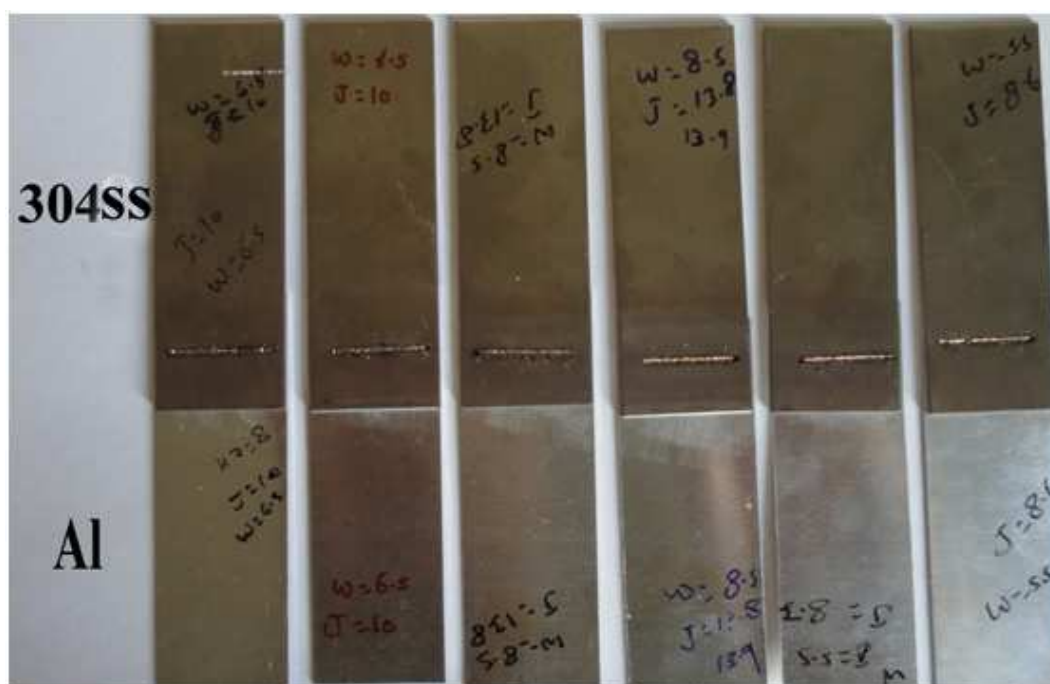
Fig. 1: Aluminum to 304 stainless steel overlap joints
