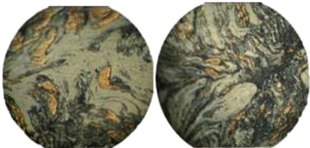
Fig. 13 Micrograph longitudinal cross sections in weld nugget at \times 100
