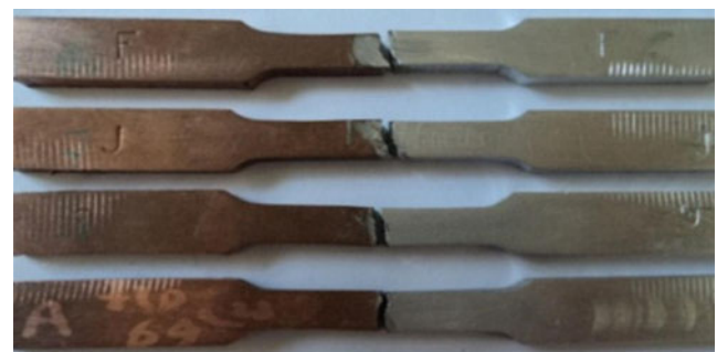
Fig. 9 Tensile test specimen after fracture for Al–Cu joint
