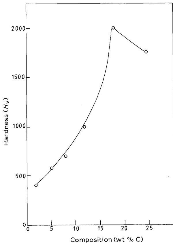
Figure 3 Variation of hardness with C content, at 800 W laser power, 3 mm beam diameter and 0.5 s pulse time.
