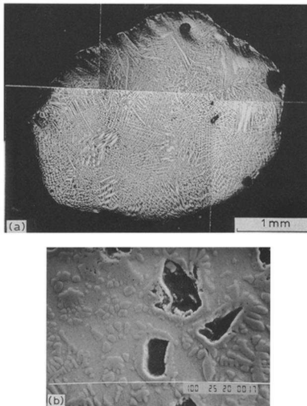
Figure 1 (a) Optical macrograph showing pellet produced from a mixture of Ti-4% C at 800 W laser power, 3 mm beam diameter and 0.5 s pulse time, and (b) SEM micrograph showing some undissolved graphite and nucleation of dendrites at the graphite-matrix interface and within the matrix.
