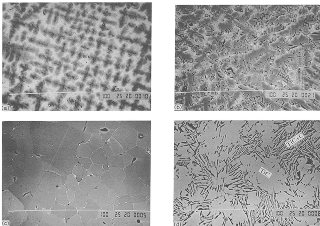
Figure 2 SEM-backscattered imaging micrographs showing the microstructures of pellets for different C contents: (a) 5 wt%, (b) 9 wt%, (c) 14 wt% and (d) 25 wt%.
