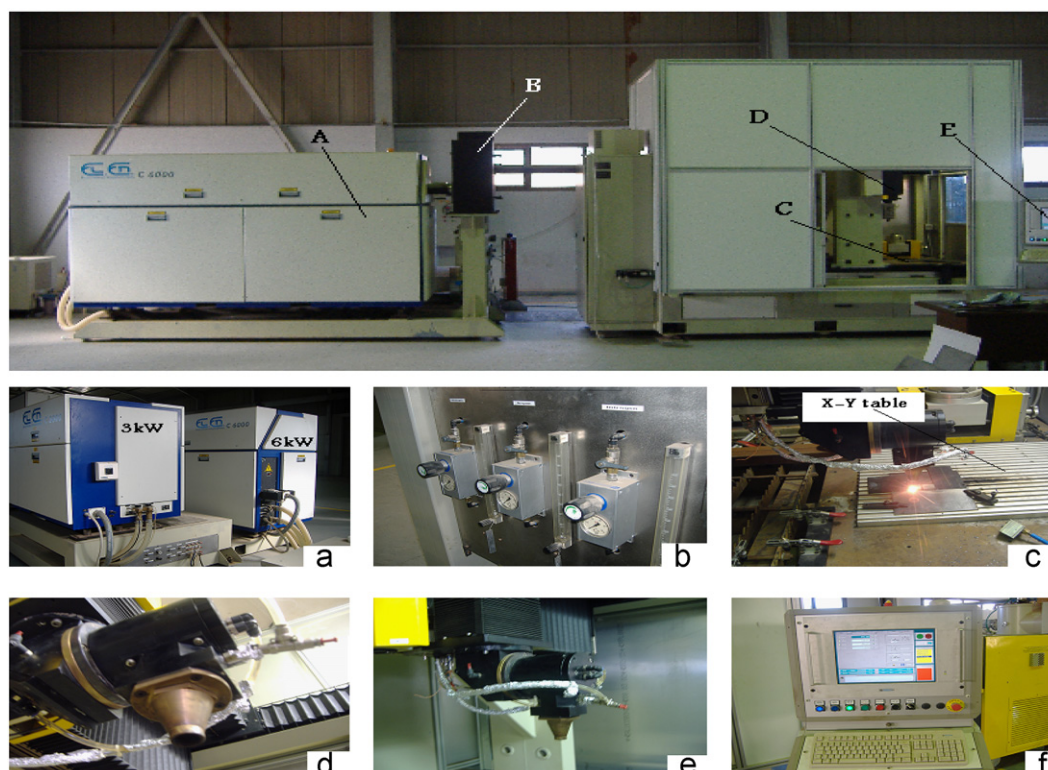
Fig. 2. Laser system: (a) CO 2 laser, (b) gas control valves, (c) X–Y table, (D) laser focus head, and (E) laser control unit.
