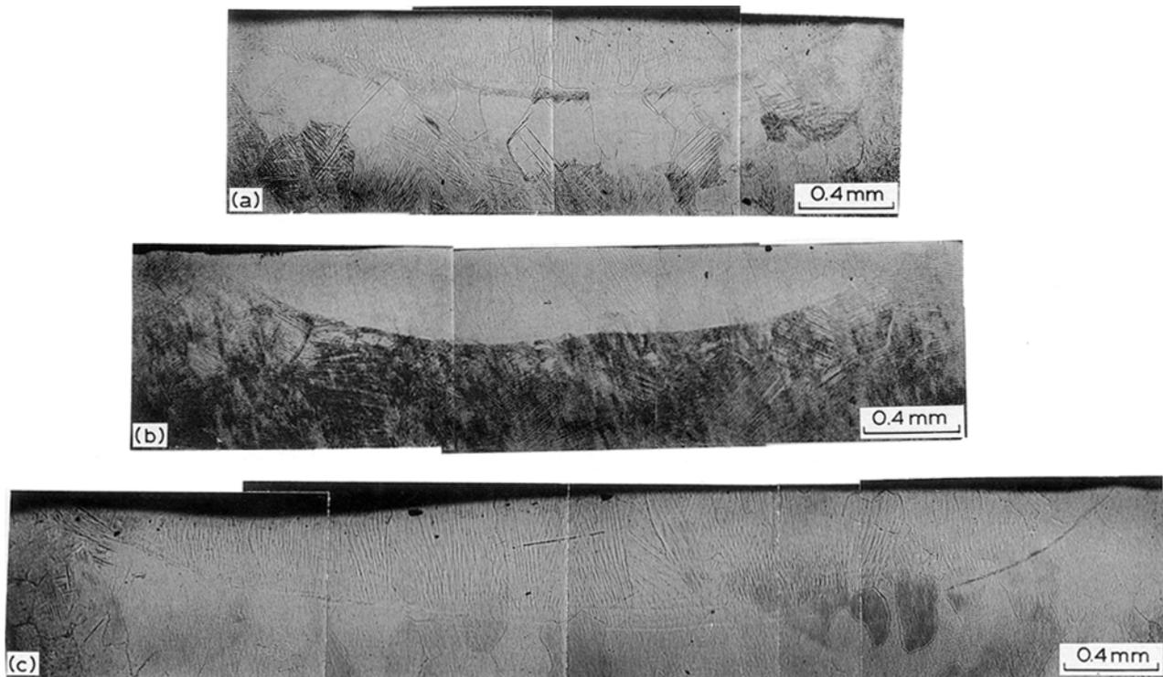
Figure 3 Optical micrographs showing transverse sections of laser-melted zones processed at 5 mm beam diameter, 8.1 mm s<sup>-1</sup> traverse speed and power (a) 3.5 kW, (b) 4 kW and (c) 4.5 kW.
