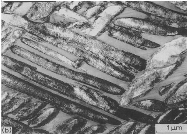
Figure 1 Microstructure of the Ti-10-2-3 alloy as-received: (a) optical microscopy and (b) TEM bright-field micrograph.
