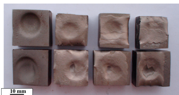
Fig. 11. Photograph showing the worn surface of the as received and TIG melted. From the left, the top samples are the as received and TIG melted samples at current 200 A, 150 A, and 100 A, respectively eroded at 90° and the lower are the as received and TIG melted samples (200 A, 150 A, and 100 A) eroded at 30°.
