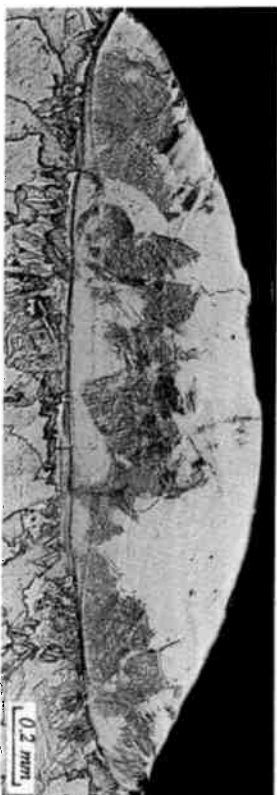
Figure 1: Example of Ti substrates laser surface alloyed with Al.
