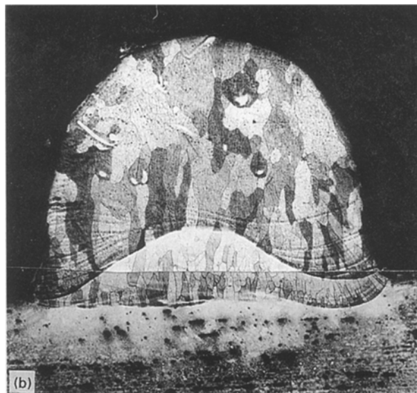
Figure 4 Optical macrographs of transverse sections of functionally graded Fe-Al coatings produced at 1.8 kW, 3 mm, 7 mm s -1 and 0.183 g s -1 Fe and various Al powder flow rates (0.032 to 0.1 g s -1 ); (a) single layer; (b) two-layer FG coating; (c) three-layer FG coatings.
