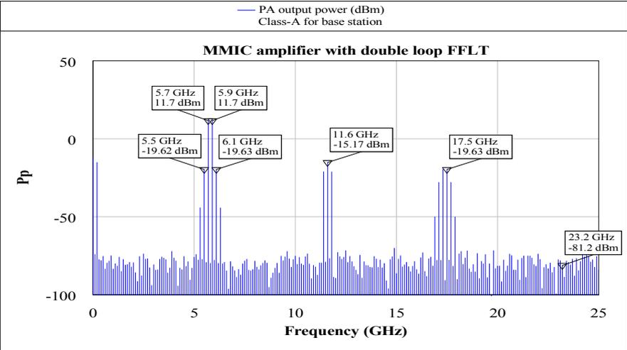
Figure 11. The two-tone test power spectrum of the main amplifier in the proposed double loop FFLT with input power level of -3.98 dBm.
