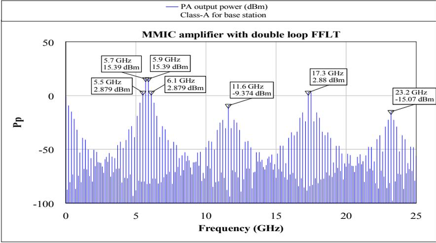
**Figure 14. The two-tone test power spectrum of the main amplifier in the proposed double loop FFLT with input power level of 5.55 dBm.**
