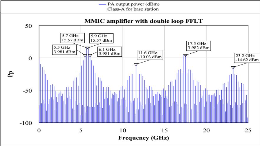
Figure 17. The two-tone test power spectrum of the main amplifier in the proposed double loop FFLT with input power level of 7.4 dBm.
