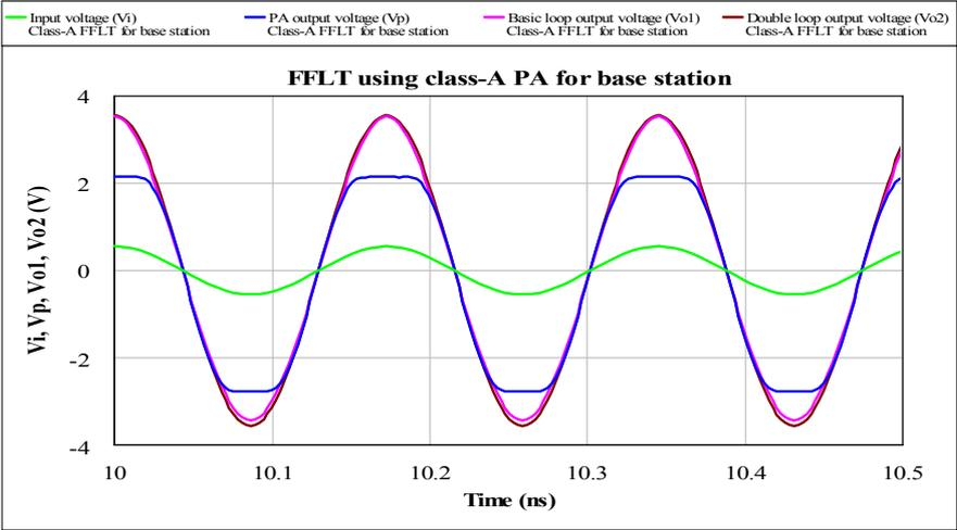
**Figure 8. The voltage waveforms of the proposed double loop FFLT with input voltage of 0.55V (peak value).**
