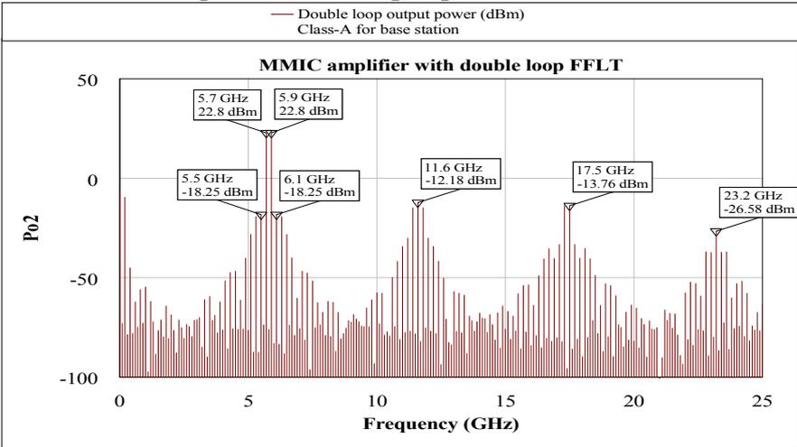
Figure 19. The two-tone test power spectrum of the second loop in the proposed double loop FFLT using class-A power amplifiers with input power level of 7.4 dBm.
