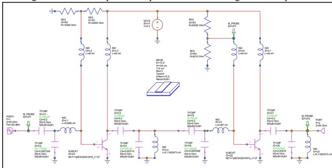
**Figure 3. The circuit schematic of class-A PA.**
