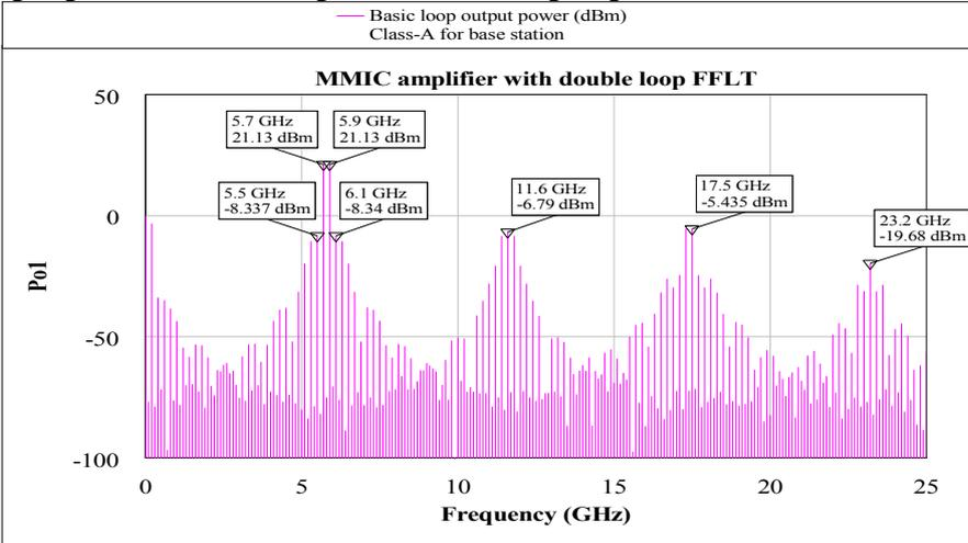
Figure 18. The two-tone test power spectrum of the basic loop in the proposed double loop FFLT with input power level of 7.4 dBm.
