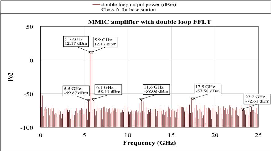
**Figure 13. The two-tone test power spectrum of the second loop in the proposed double loop FFLT with input power level of -3.98 dBm.**
