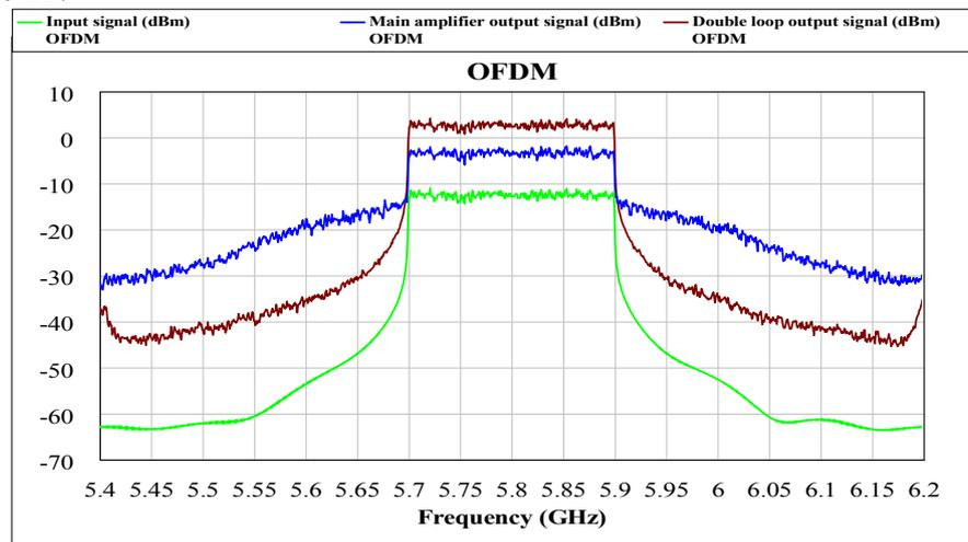
**Figure 21. The OFDM response of the proposed double loop FFLT.**
