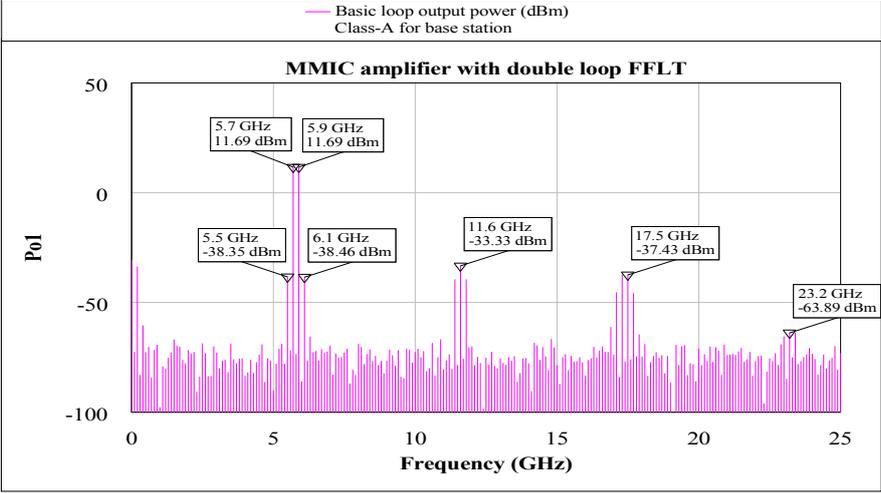
Figure 12. The two-tone test power spectrum of the basic loop in the proposed double loop FFLT with input power level of -3.98 dBm.
