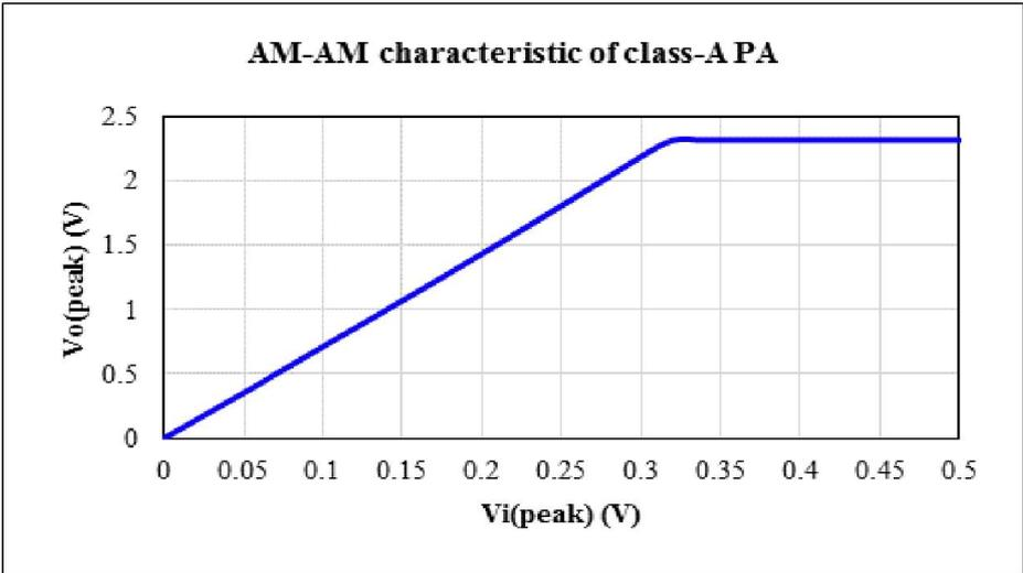
Figure 6. AM-AM characteristics of the proposed class-Aerror amplifier.
