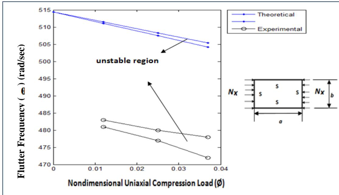
Figure 16. Theoretical and experimental effects of loading on primary instability region of SSSS plate.
