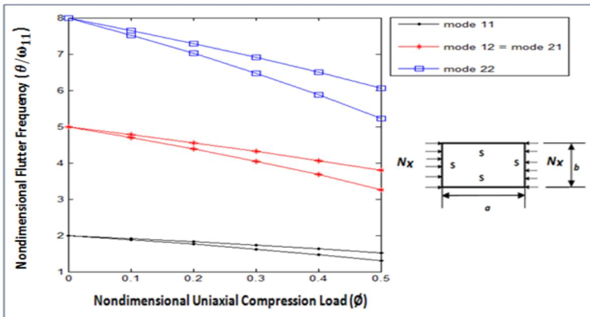
Figure 11: Effect of nondimensional uniaxial compression load on primary instability region of SSSS plate,  $a/b = 1$  and  $\delta = 0.3$ .
