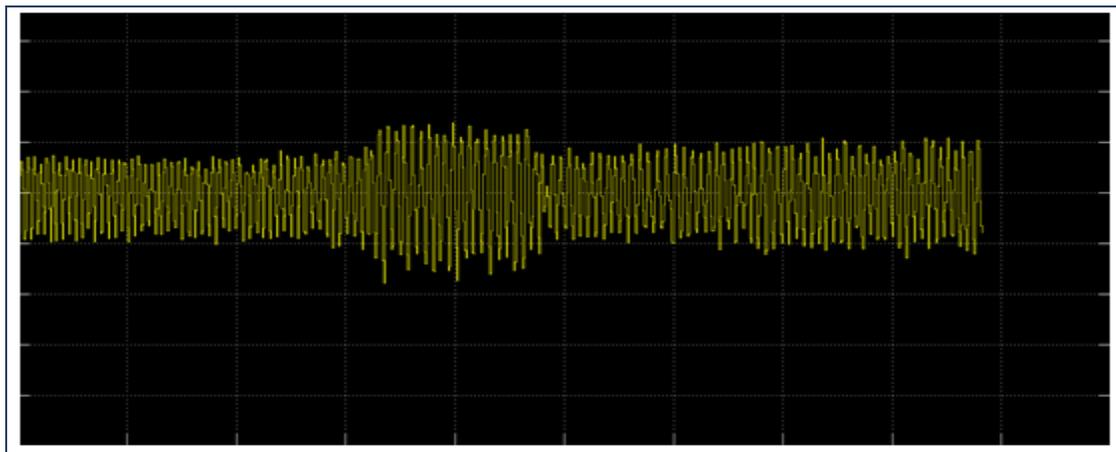
Figure 17. Acceleration curve for dynamic instability with loading ( $\phi = 0.012$ ).
