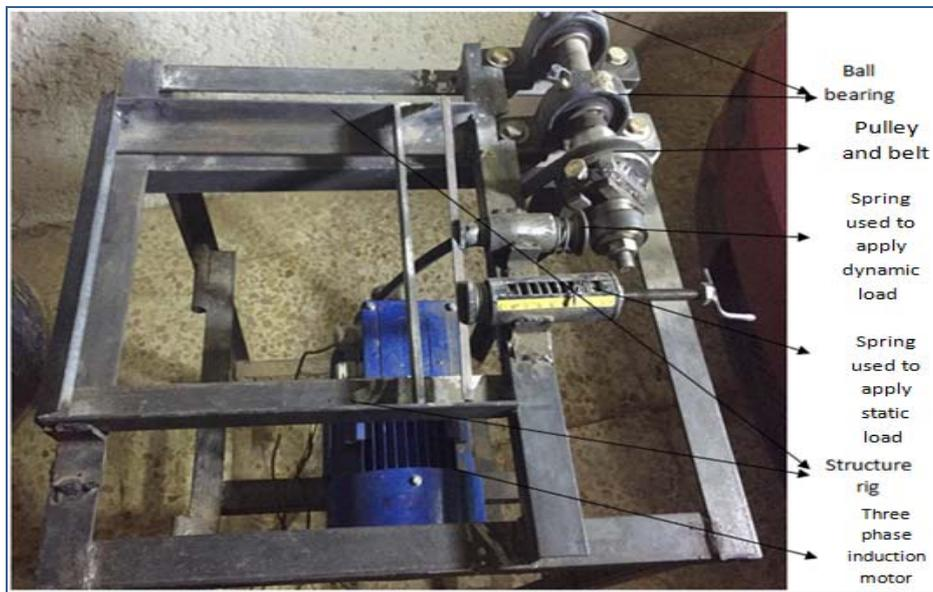
Figure 2. Exciter used in vibration and stability test.
