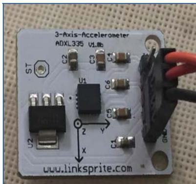
Figure 3. Accelerometer.
