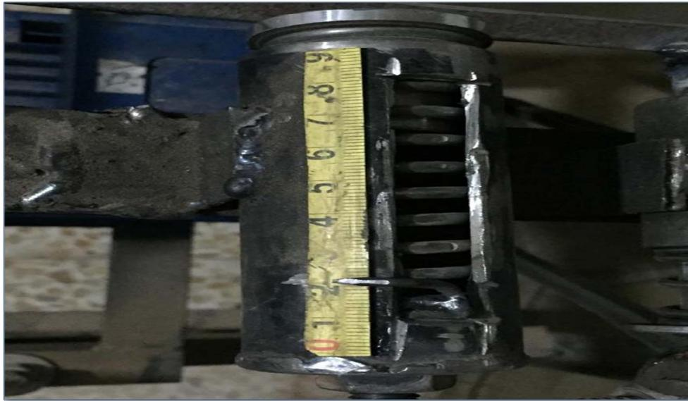
Figure 5: Spring used to apply static load
