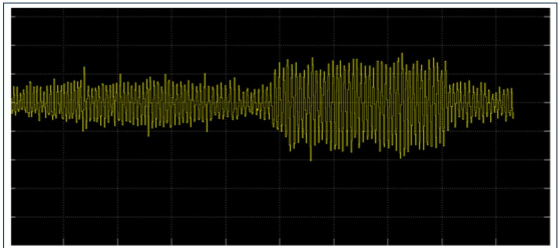
Figure 15. Acceleration curve for dynamic instability with excitation parameter ( $\delta = 0.433$ ).
