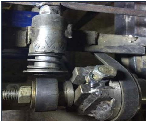
Figure 6: Shaft connected in slot used to apply dynamic load
