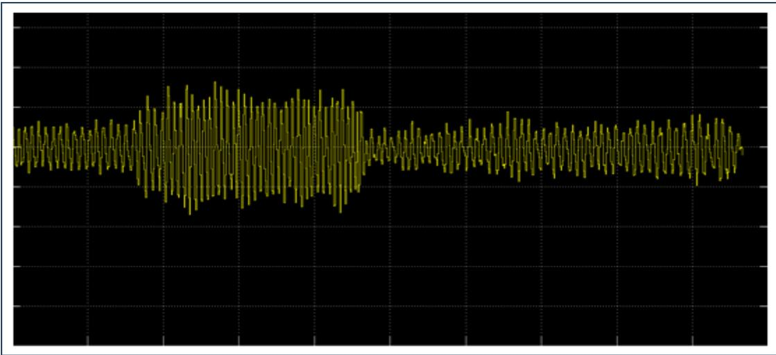
Figure 14. Acceleration curve for dynamic instability with excitation parameter ( $\delta = 0.288$ )
