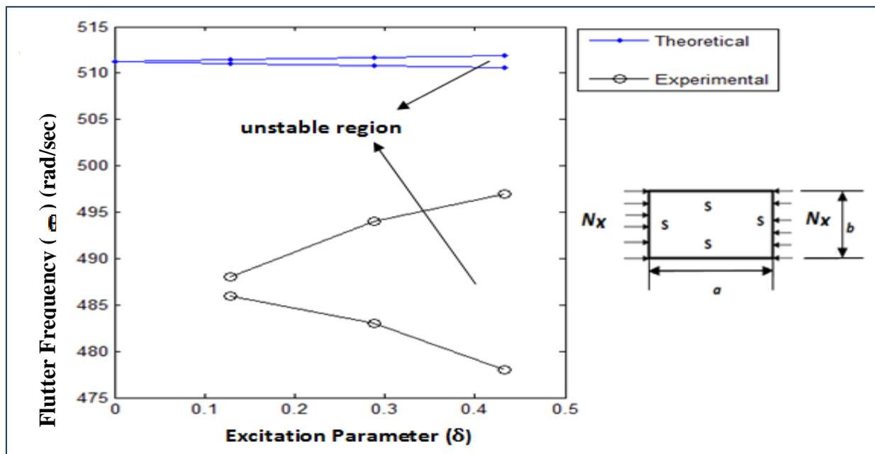
Figure 12. Theoretical and experimental effects of excitation parameter on primary instability region of SSSS plate.
