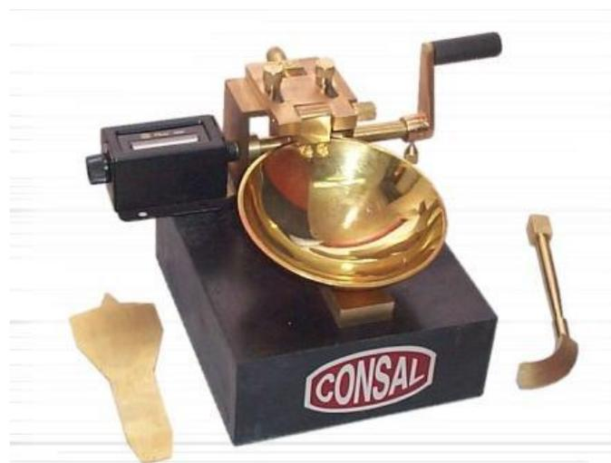
Figure (5) show the mechanical device used to calculate LL.
