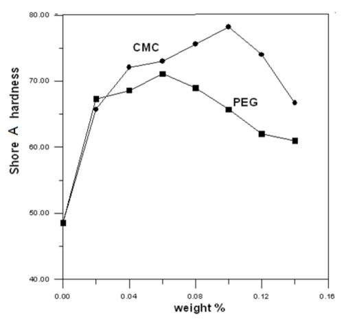
Fig. (2): relationship between Shore A hardness and the weight fractions of CMC and PEG4000.
