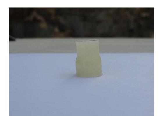
Fig.(9): the shape of failure of epoxy specimen reinforced with 0.04 wt% of PEG after compression test.
