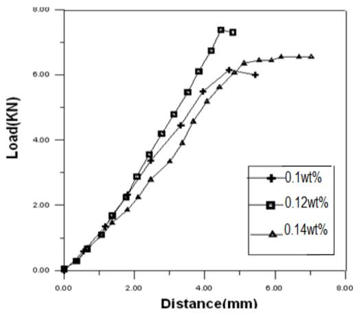
Fig.(4): data of compression for epoxy specimens reinforced with CMC (0.1-0.14) wt %.
