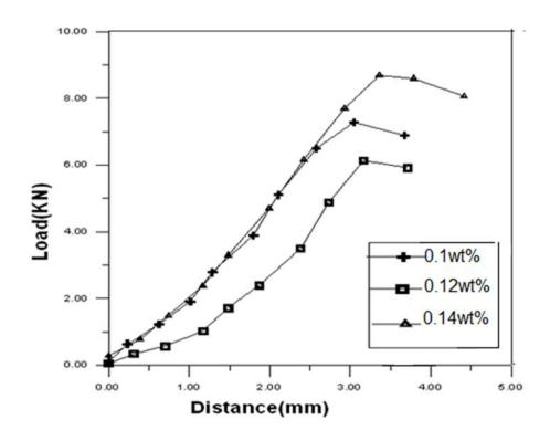
Fig.(8): data of compression test for epoxy specimens reinforced with PEG (0.1-0.14) wt %
