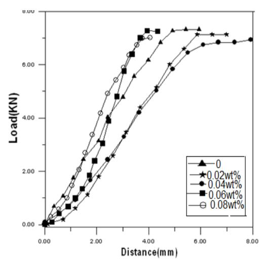
Fig.(3): data of compression test for epoxy specimens reinforced with CMC (0.02-0.08) wt %.
