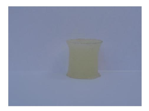
Fig.(6): the shape of failure of epoxy specimen reinforced with 0.12 wt % of CMC after compression test.
