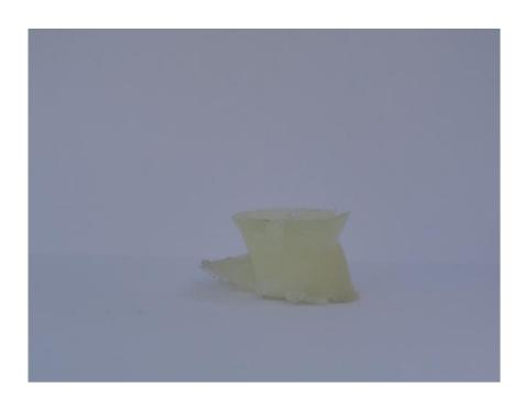
Fig.(5): the shape of failure of unreinforced epoxy specimen after compression test.
