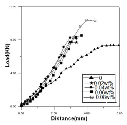
Fig.(7): data of compression test for epoxy specimens reinforced with PEG (0.02-0.08) wt %
