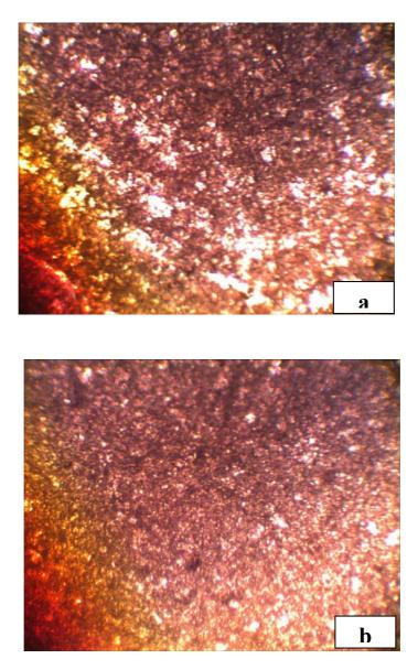
Fig. 4: light optical micrograph for as polished aluminum reinforced by 12wt.%  $\alpha$ -Al<sub>2</sub>O<sub>3</sub> particles (a) before sintering process, (b) after sintering process Alumina particles appear darker than the aluminum matrix.
