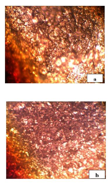
Fig. 3: light optical micrograph for as polished aluminum reinforced by 6 wt.%  $\alpha$ -Al<sub>2</sub>O<sub>3</sub> particles (a) before sintering process, (b) after sintering process Alumina particles appear darker than the aluminum matrix.
