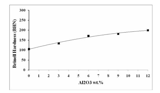
Fig. 5:Illustrate the relation between concentration of  $\alpha$ -alumina particles and Brinell hardness (BHN).
