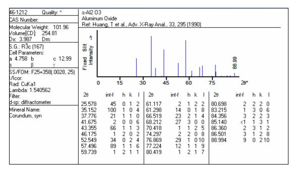
Fig. 2: Standard Diffractograms of α-Al<sub>2</sub>O<sub>3</sub>
