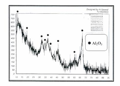
Fig. 1: Diffractograms from the surface of α-(Al<sub>2</sub>O<sub>3</sub>) particles.
