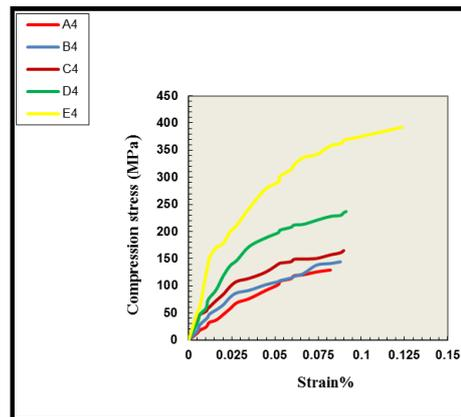
**Figure 4.** Compression stress-strain curve for alloys A4, B4, C4, D4 and E4 which compacted at 450 MPa and sintered at 850°C for 9hours.
