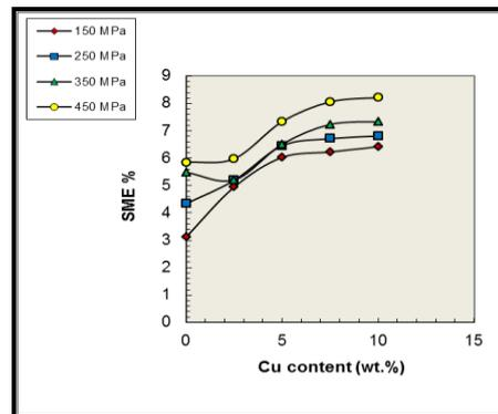
**Figure 14.** Effect of copper content on SME properties obtained from compression test at RT.
