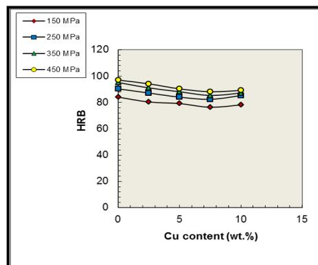
**Figure 2.** HRB Vs copper content for alloy A, B, C, D and E compacted at different compacting stress.
