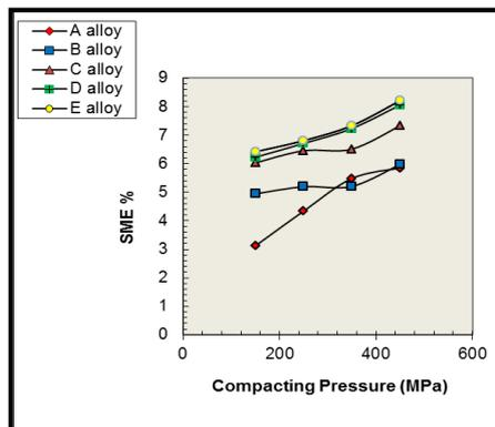
**Figure 11.** Effect of compacting pressure on SME properties obtained from compression test at RT (room temperature).
