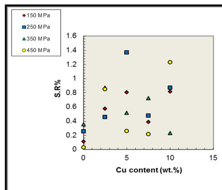
**Figure 13.** Effect of copper content on strain recovery properties obtained from compression test at RT.
