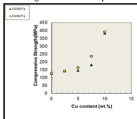
**Figure 5.** Compressive strength as a function of Cu content for A, B, C, D and E alloys which compacted at 350 MPa and 450 MPa and sintered at 850°C for 9 hours.
