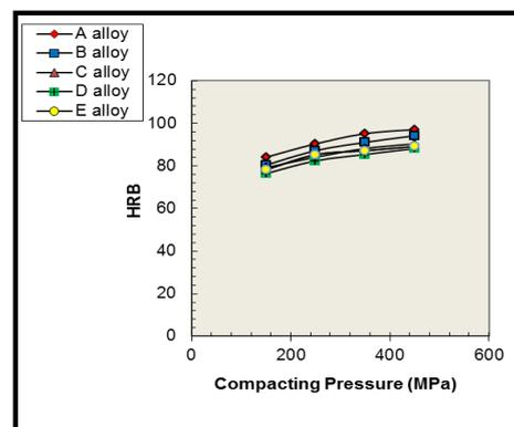
**Figure 1.** Effect of compacting pressure on the HRB values for alloy A, B, C, D and E sintered at 850°C for 9 hours.
