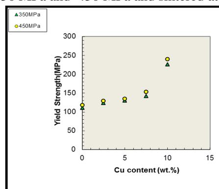
**Figure 6.** Yield strength as a function of Cu content for A, B, C, D and E alloys that compacted at 350 MPa and 450 MPa and sintered at 850°C for 9 hours.
