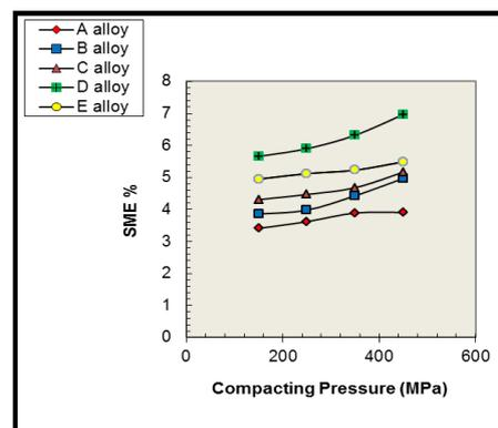
**Figure 9.** Effect of compacting pressure on SME properties obtained from Hardness test.
