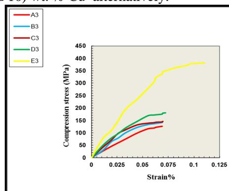
**Figure 3.** Compression stress-strain curve for alloys A3, B3, C3, D3 and E3 which compacted at 350 MPa and sintered at 850°C for 9 hours.
