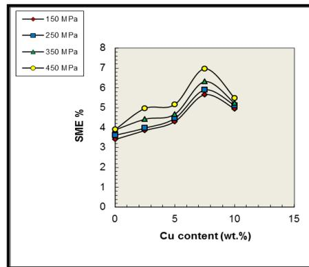
**Figure 10.** Effect of copper content on SME properties obtained from Hardness test.
