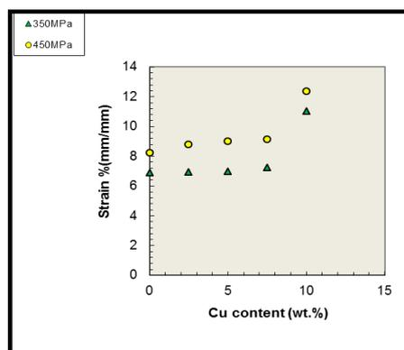
**Figure 8.** Strain as a function of Cu content for A, B, C, D and E alloys that compacted at 350 MPa and 450 MPa and sintered at 850°C for 9 hours.
