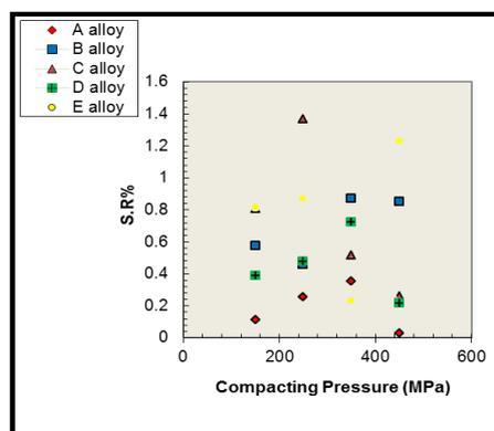
**Figure 12.** Effect of compacting pressure on strain recovery properties obtained from compression test at RT.
