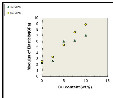
**Figure 7.** Modulus of elasticity as a function of Cu content for A, B, C, D and E alloys which compacted at 350 MPa and 450 MPa and sintered at 850°C for 9 hours.
