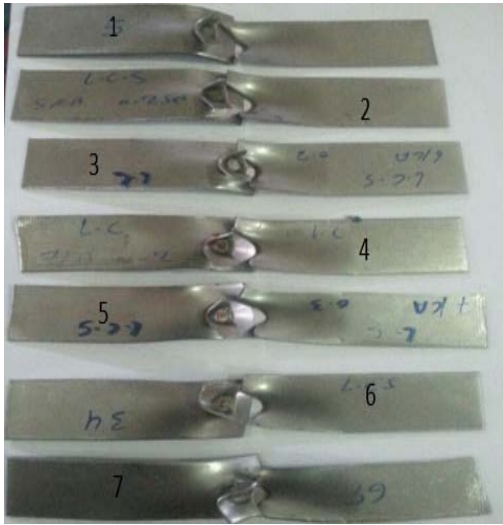
Fig. 13: The failure mode of shear test
