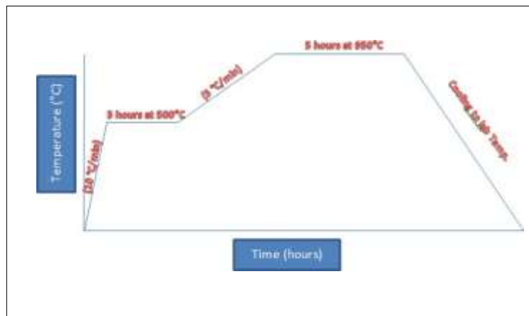
Fig. 2: The heat treatment process for coated sample.
