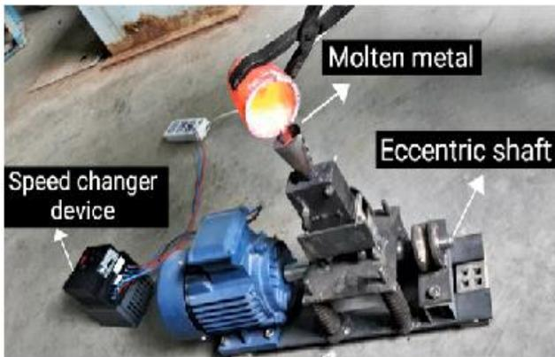
Figure 1. Vibration device [9].
