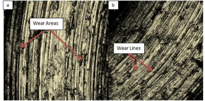
Figure 6. Microstructure for S2 alloy magnification at 100X after wear test under load of 20 N for 25 minute: a) at 27 °C b) at 100 °C.
