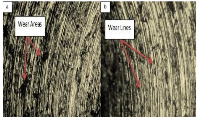
Figure 7. Microstructure for S3 alloy magnification at 100X after wear test under a load of 20 N for 25 minute: a) at 27 °C b) at 100 °C.
