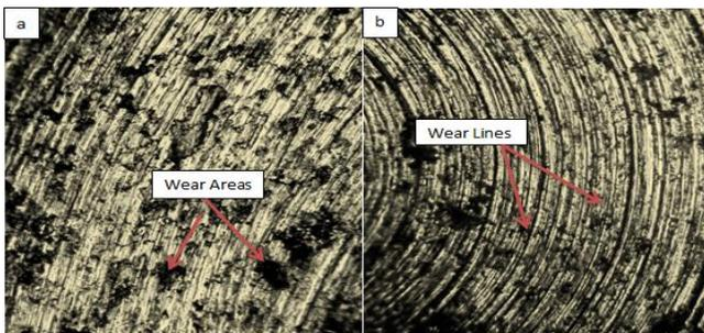
Figure 5. Microstructure for S1 alloy magnification at 100X after wear test under a load of 20 N for 25 minute: a) at 27 °C b) at 100 °C.
