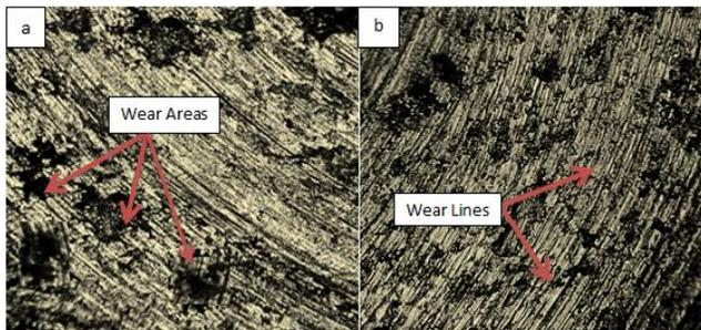
Figure 4. Microstructure for S0 alloy magnification at 100X after wear test under a load of 20 N for 25 minute: a) at 27 °C b) at 100 °C.
