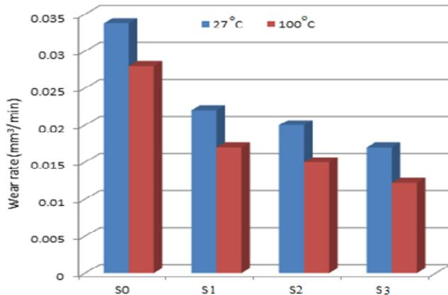
Figure 3. Wear rate of the prepared samples under a load of 20 N for 25 minutes.
