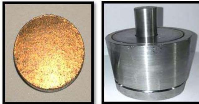
**Figure 3:** a- Types of Prepared Samples, b-Steel Die Used at Present Study.
