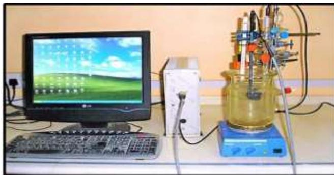
**Figure 5 :** Tafel Instruments for Polarizations Test.
