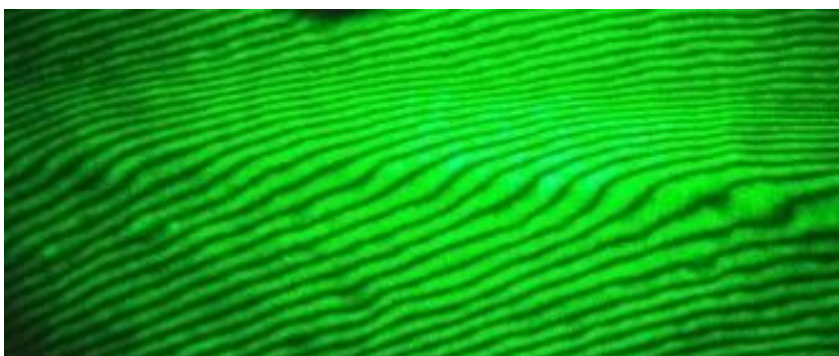
Figure 2: NiO thickness measurement via the interference Tolansky method
