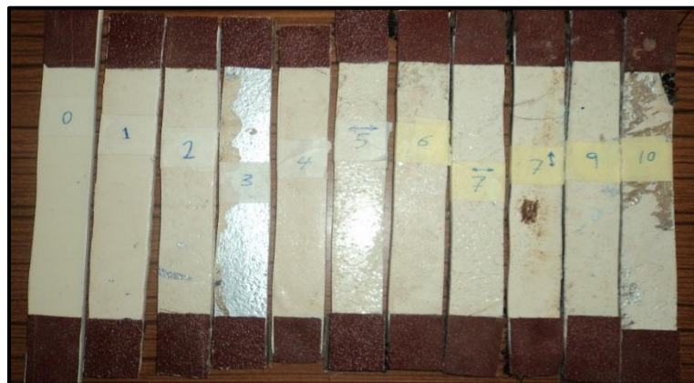
Figure (4): Experimental tensile Specimen, (ASTM D3039).
