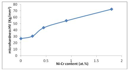
Fig. 5: Effect of content Ni-Cr at.% on Vickers microhardness of aluminum. Refrences
