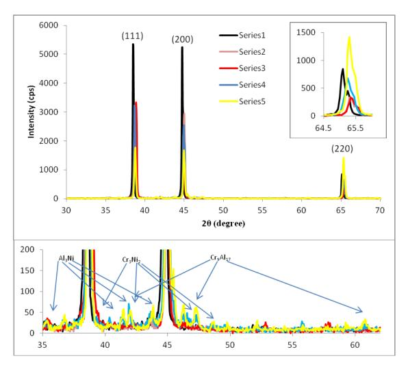
Fig. 3:XRD pattern of Al and Al-Ni-Cr alloys.
