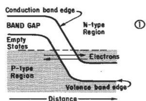
Electrons at same level on both sides of junction. No net current.
