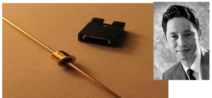
1N3716 tunnel diode (with jumper for scale)
