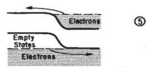
Electrons raised until they spill over barrier. Current increases.
