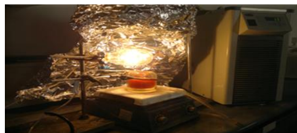
Figure.3. Main parts of the photocatalytic cell used in Photocatalytic degradation of prepared azo dye
