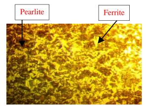
Fig.7; Microstructure of normalizing (80x)
