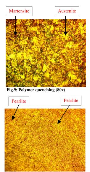
Fig.11; Polymer tempering (80x)
