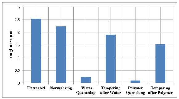
Figure 5; Roughness for untreated and heat treated samples
