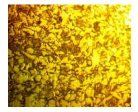
Fig.18; Oil quenching at (80x)
