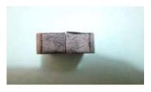
Fig.3; Sample after impact strength test
