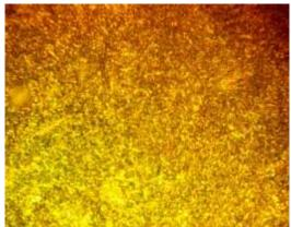
**Fig.12**; Water tempering at 400°C with (80x)
