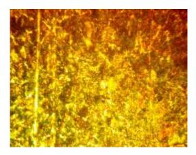
**Fig.20**; Oil tempering at 400°C with (80x)
