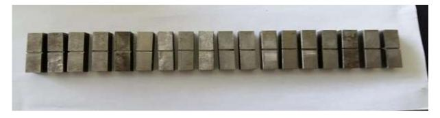
Fig. 1; Impact strength samples before heat treatment
