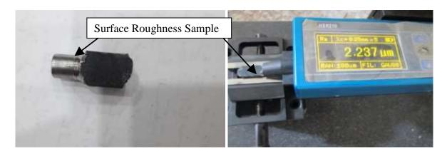
Fig. 4; Sample of surface roughness test
