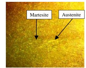
Fig.11; Water Tempering at 200°C with (80x)
