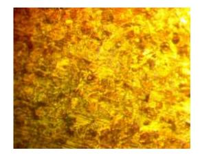
Fig.19; Oil tempering at 200°C with (80x)
