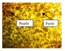
**Fig.9;** Microstructure with air cooling (80x)
