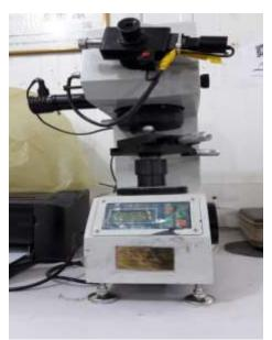
Fig. 7; Microhardness Tester
