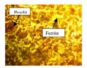
Fig.8; Microstructure of non-heat treated (80x)
