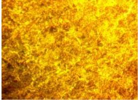
Fig.21; Oil tempering at 600°C with (80x)
