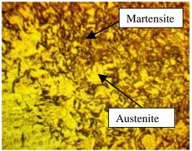
Fig.10; Water quenching with (80x)
