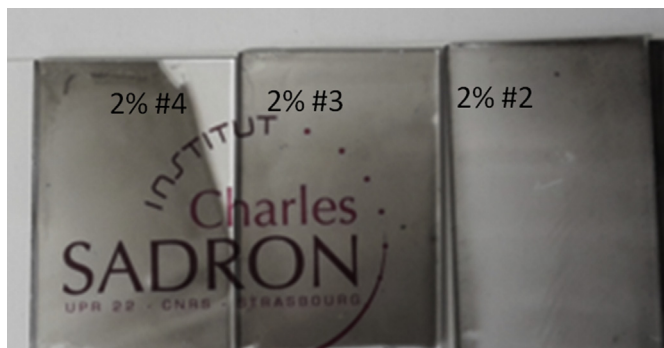
Fig. 2. 2 wt.% PMMA-grafted-MWCNT/PMMA coating of 15–20 \mu\text{m} on glass substrate obtained by Doctor Blade technique (samples with different monomer:MWCNT-Br ratio (wt.:wt.); monomer:CuBr:PMDETA ratio (mol:mol:mol) and monomer:solvent ratio (v:v) see Table 1 type #2, #3, #4).
